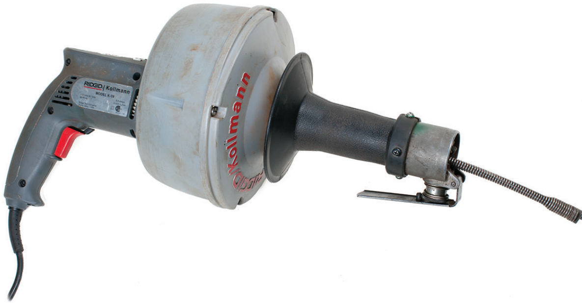
Figure 5 Drain auger powered by an electric drill. (Skilled Trades BC, 2021) Used with permission.
