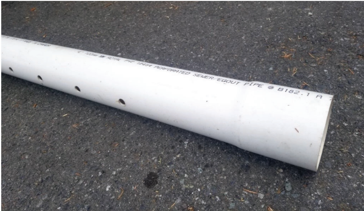
Figure 4 Perforated PVC pipe. (Rod Lidstone) CC BY ( https://creativecommons.org/licenses/by/4.0/deed.en )
