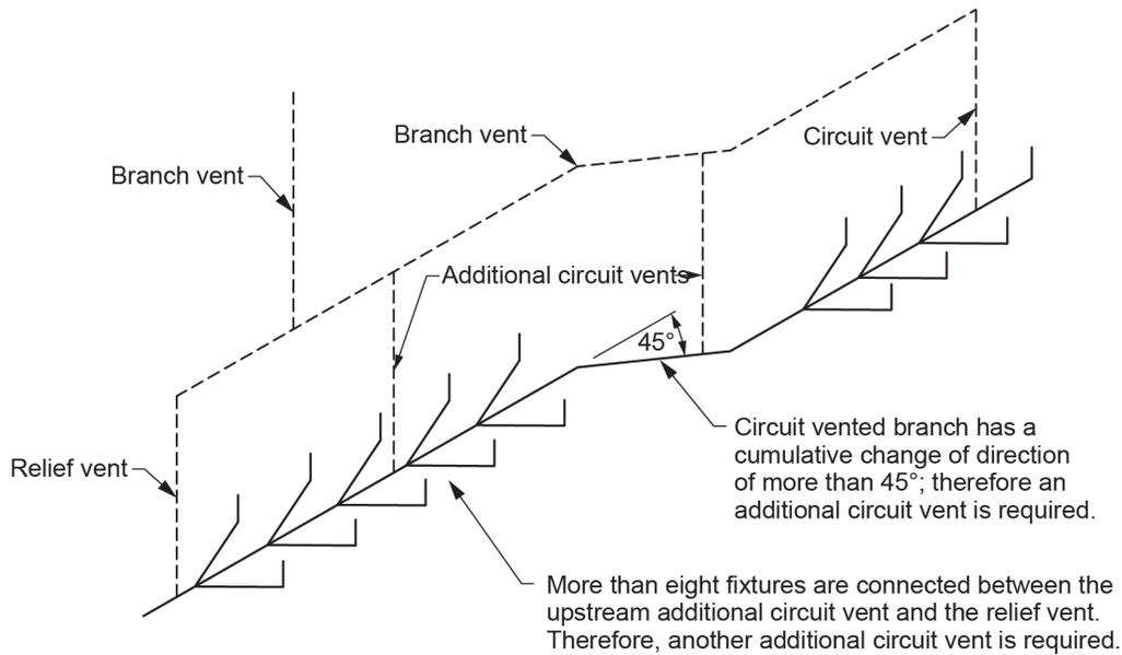
**Figure 17** Circuit-vented branch showing the requirements for additional circuit vents. (Skilled Trades BC, 2021) Used with permission.
