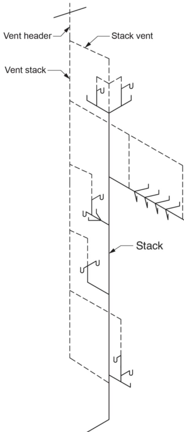
**Figure 30** Vent stack connected to a stack and becoming a vent header. (Skilled Trades BC, 2021) Used with permission.
