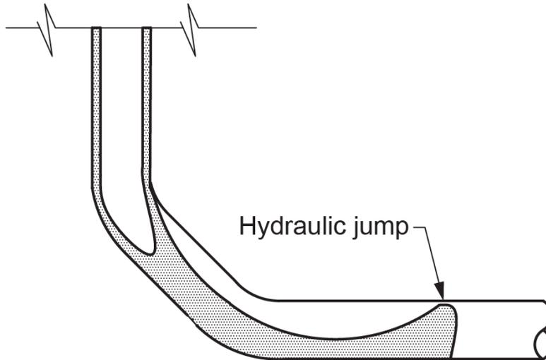
**Figure 6** Vertical to horizontal flow. (Skilled Trades BC, 2021) Used with permission.
