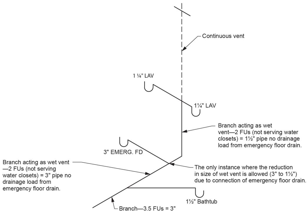
**Figure 8** A wet vent being reduced in size due to the connection of a 3 in. emergency floor drain. (Skilled Trades BC, 2021) Used with permission.
