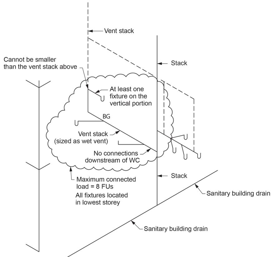
**Figure 5** Rules surrounding fixtures connecting to the base of vent stacks. (Skilled Trades BC, 2021) Used with permission.
