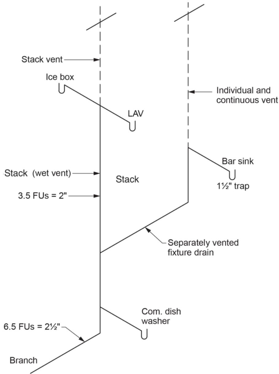
**Figure 2** Separately vented fixture draining to a multi-storey wet vent. (Skilled Trades BC, 2021) Used with permission.
