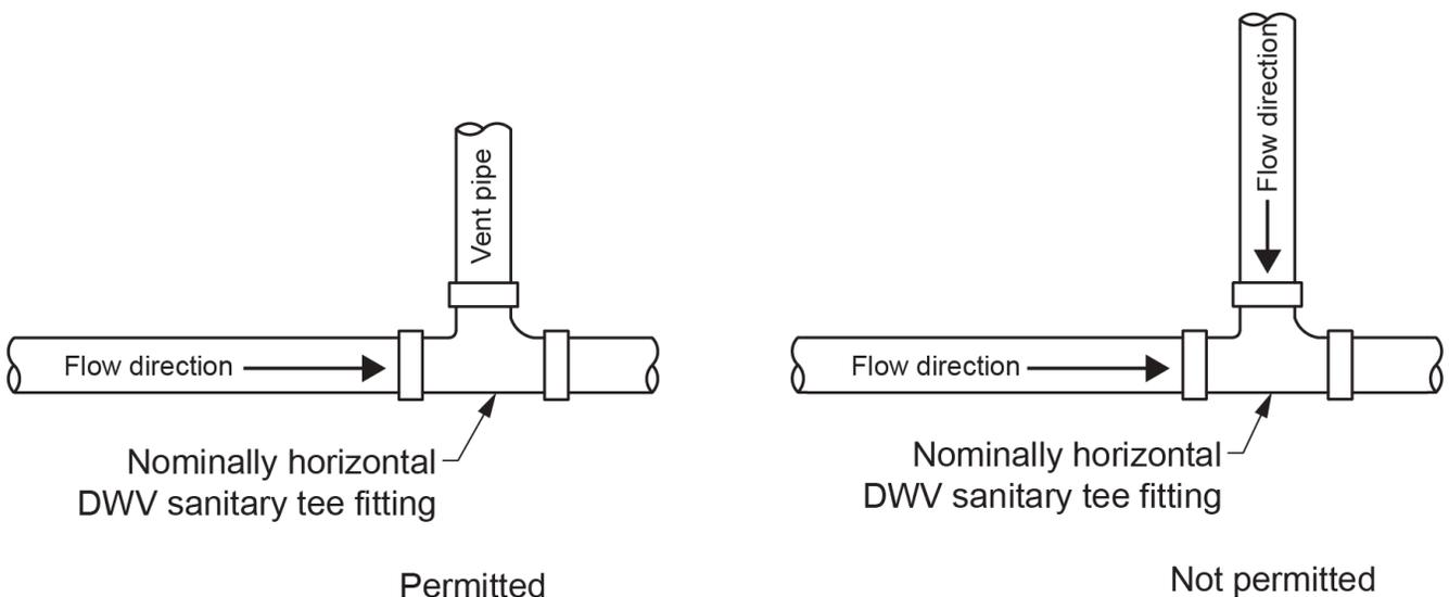
**Figure 4** NPC restrictions for single sanitary tee fittings. (Skilled Trades BC, 2021) Used with permission.
