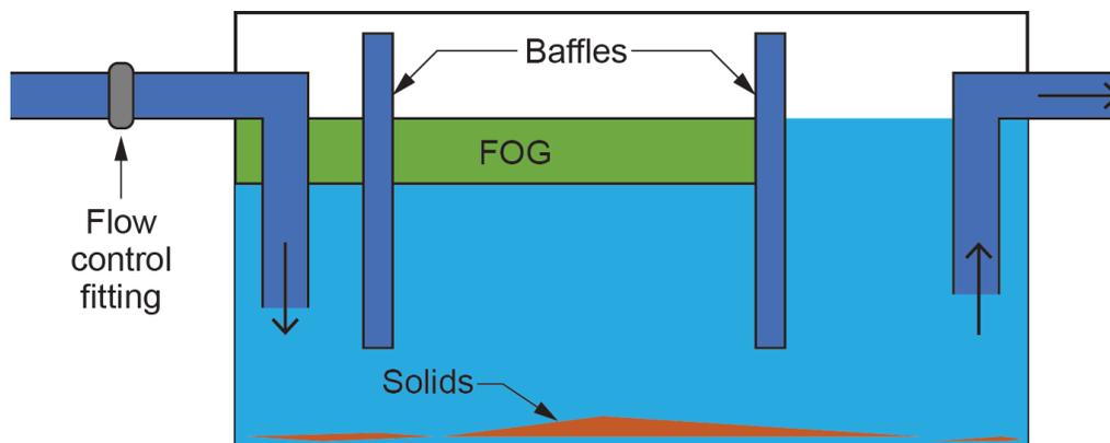
**Figure 2** Grease interceptor. (Skilled Trades BC, 2021) Used with permission.
