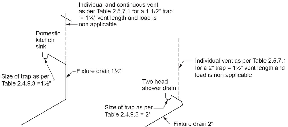
**Figure 1** Individual vent sizes based on trap size. (Skilled Trades BC, 2021) Used with permission.
