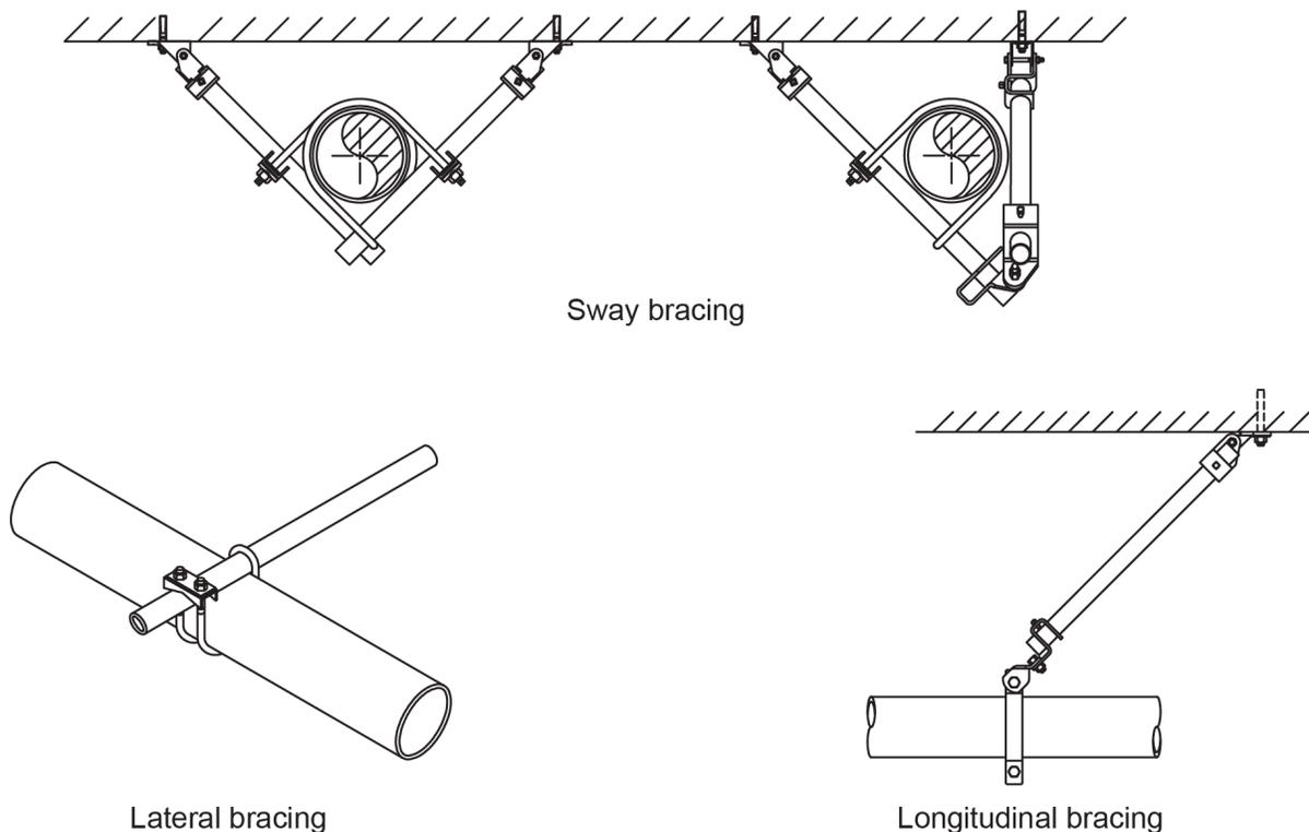
**Figure 21** Seismic restraint bracing assemblies. (Skilled Trades BC, 2021) Used with permission.
