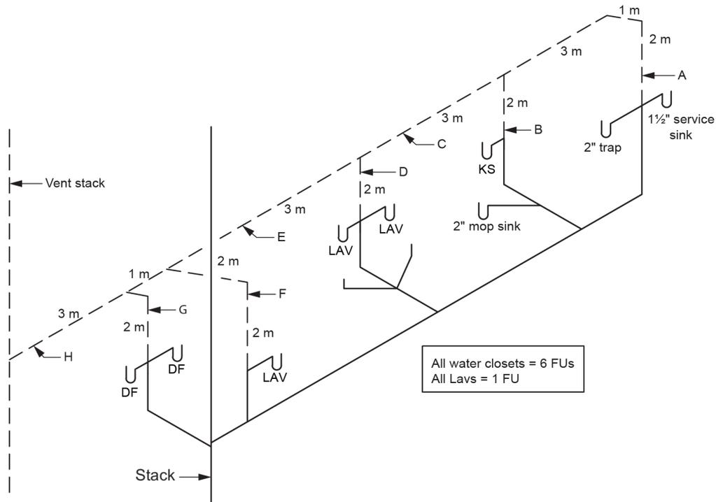
**Figure 3** Branch vent additive loads serving Category 1 vents. (Skilled Trades BC, 2021) Used with permission.
