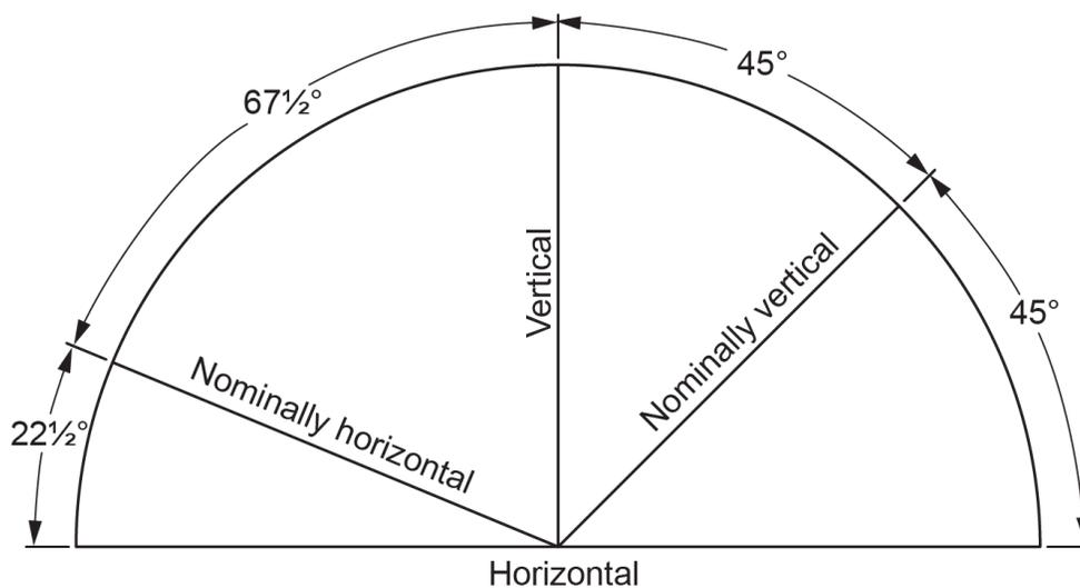
**Figure 21** Nominally horizontal and vertical. (Skilled Trades BC, 2021) Used with permission.
