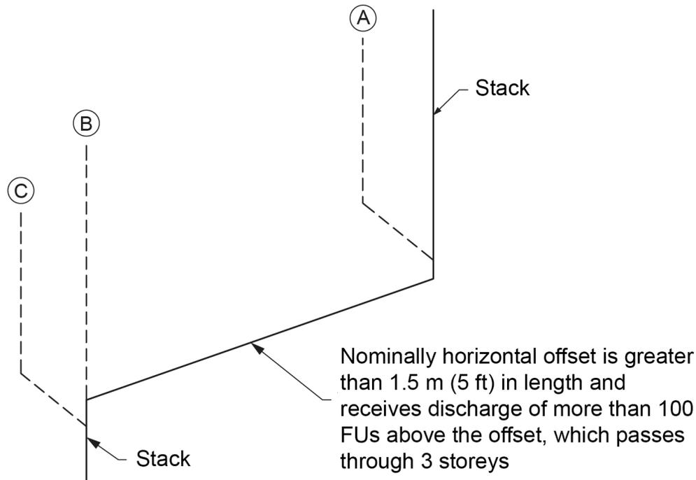
**Figure 18** Offset relief vents serving a nominally horizontal offset in a stack. (Skilled Trades BC, 2021)
