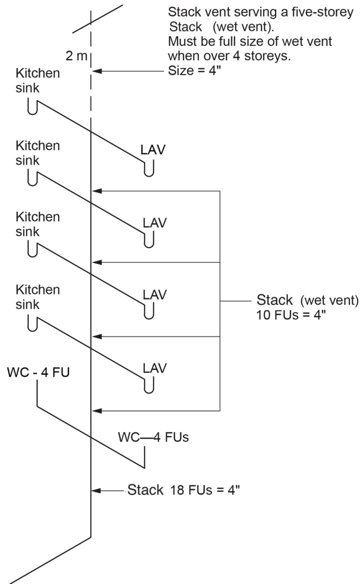
**Figure 6** Stack vent sizing when serving a stack. (Skilled Trades BC, 2021)
