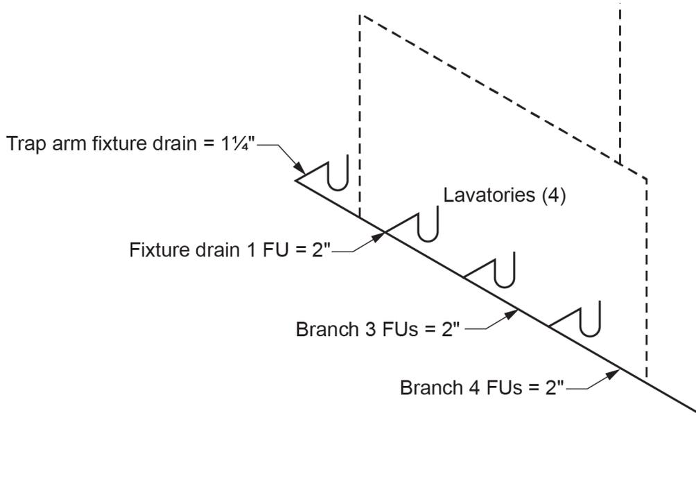
**Figure 17** Circuit-vented branch serving 1.25 in. lavatories increased to 2 in. fixture drain downstream of the circuit vent connection. (Skilled Trades BC, 2021) Used with permission.
