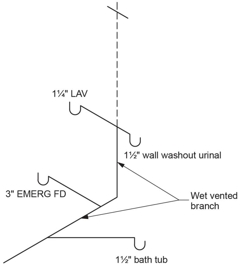
**Figure 5** Hydraulic load on a wet vent for the purpose of NPC Table 2.5.8.1. (Skilled Trades BC, 2021) Used with permission.
