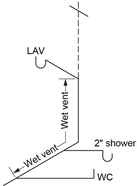
**Figure 31** Wet vent serving a bathroom group. (Skilled Trades BC, 2021) Used with permission.
