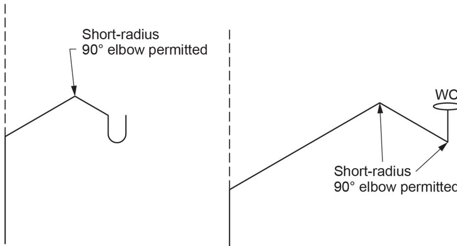
**Figure 7** NPC restriction for short-radius 90° elbows used in systems 100 mm (4 in.) in size or less. (Skilled Trades BC, 2021) Used with permission.
