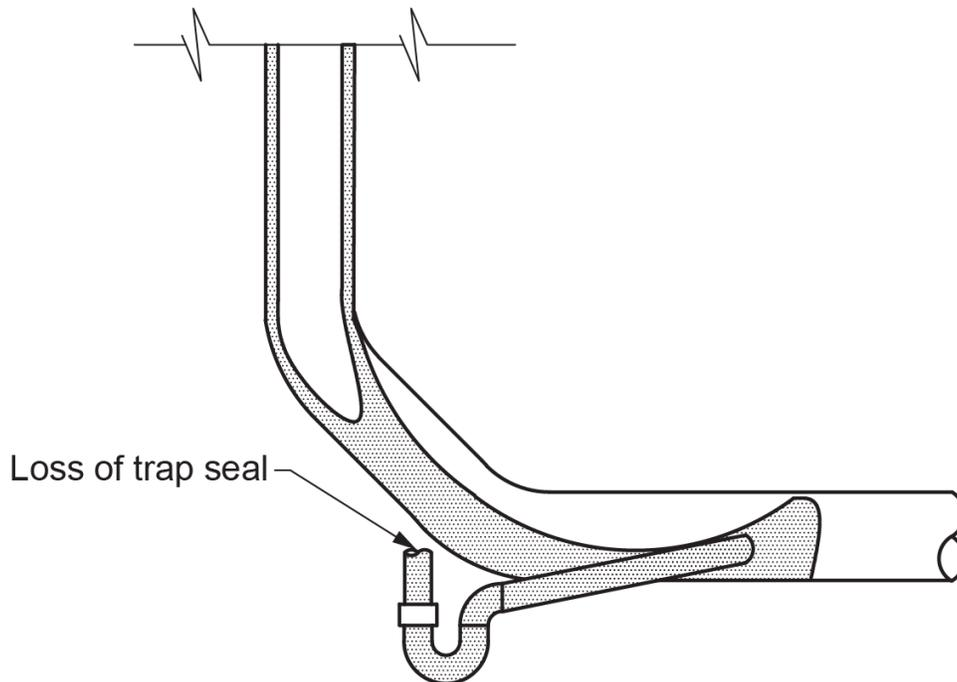
**Figure 7** Loss of trap seal. (Skilled Trades BC, 2021) Used with permission.
