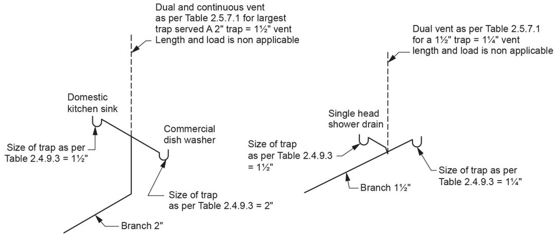
**Figure 2** Dual vents size based on largest trap size. (Skilled Trades BC, 2021) Used with permission.
