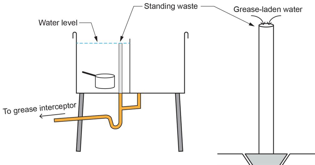
**Figure 1** Commercial pot sink with standing waste. (Skilled Trades BC, 2021) Used with permission.
