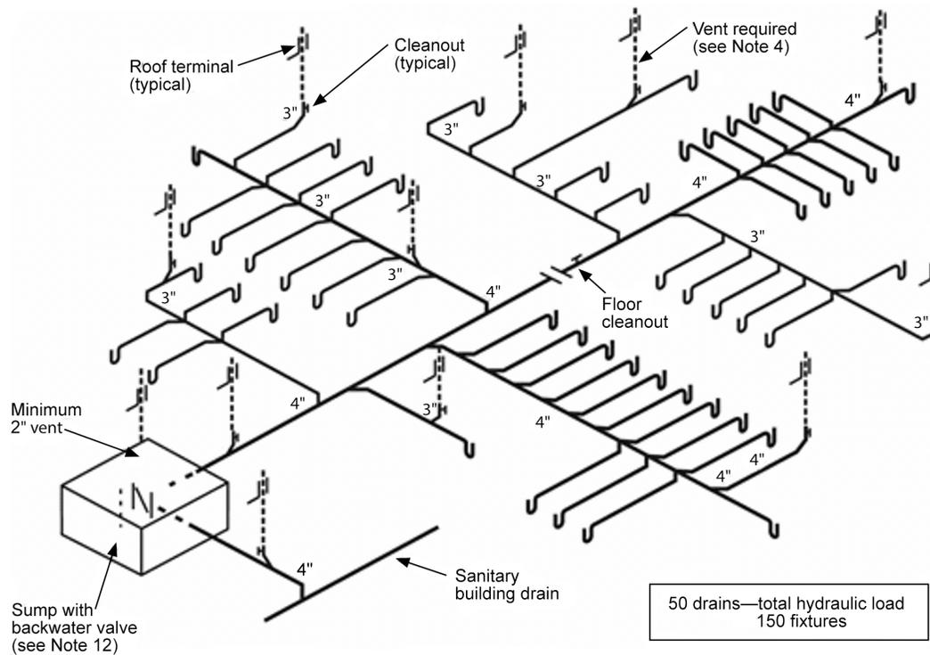
**Figure 4** Sump with backwater valve. (Skilled Trades, BC, 2007)
