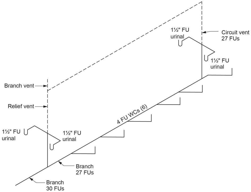
**Figure 23** The hydraulic load on a circuit vent is the connected load to the circuit-vented branch, including fixtures connected to the circuit vent. The load does not include the fixtures connected to the relief vent. (Skilled Trades BC, 2021) Used with permission.
