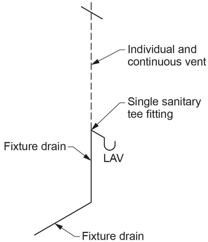
**Figure 13** Individual and continuous vent serving a single lavatory
