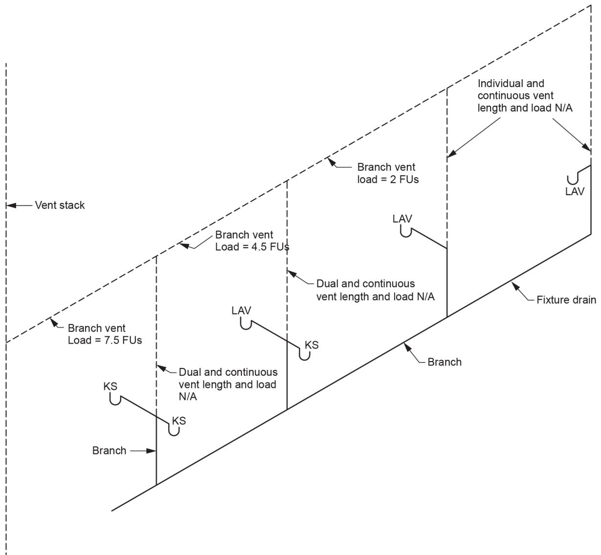
**Figure 2** Hydraulic load on certain branch vent sections. (Skilled Trades BC, 2021) Used with permission.
