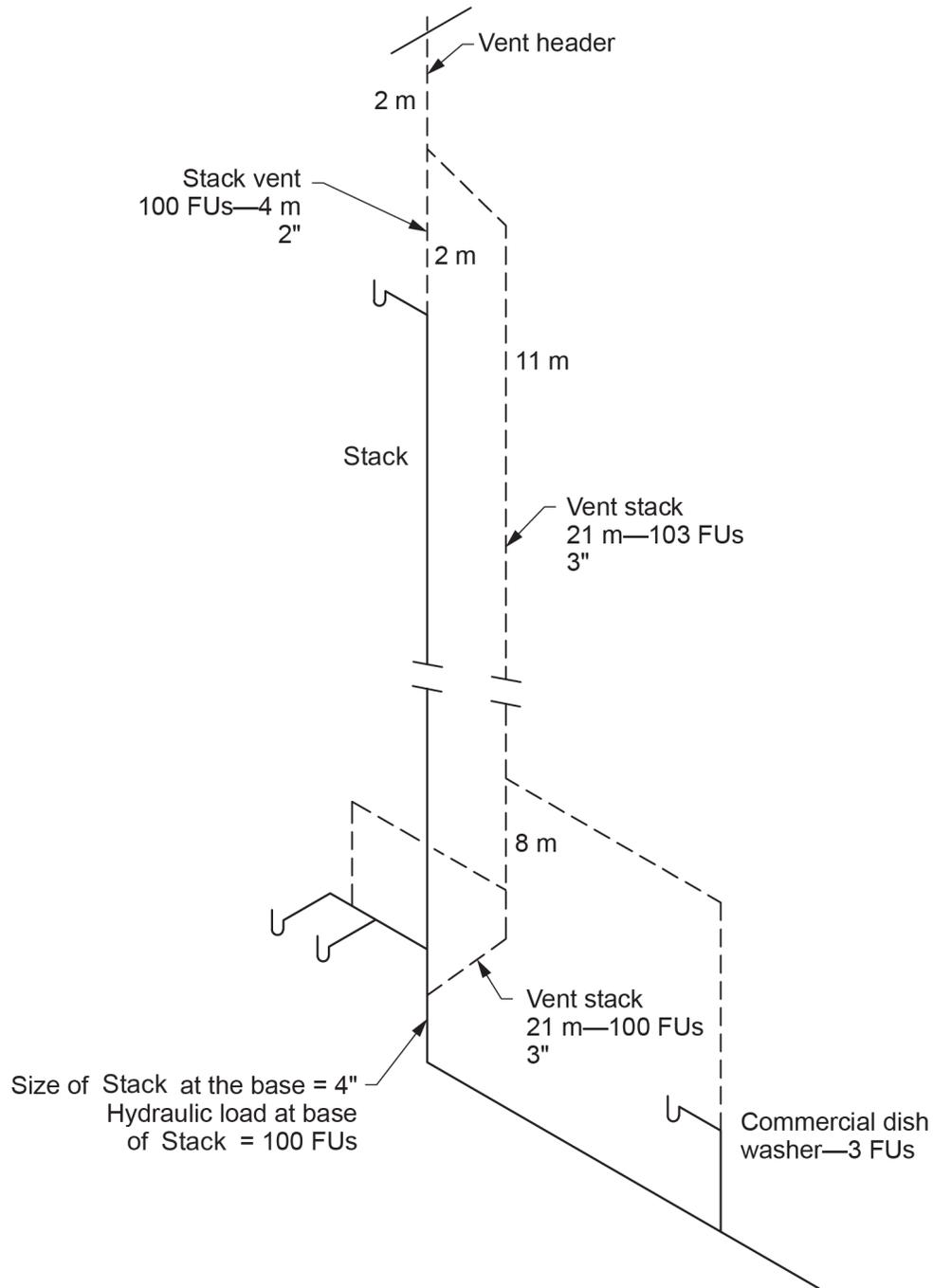
**Figure 4** Vent stack hydraulic load determination. (Skilled Trades BC, 2021) Used with permission.
