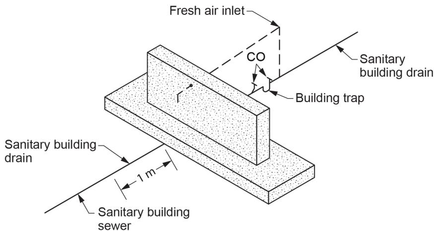
**Figure 9** Building drain and building sewer with building trap. (Skilled Trades BC, 2021) Used with permission.
