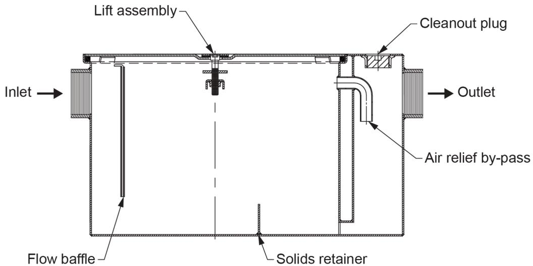
**Figure 20** Commercial-grade grease interceptor. (Skilled Trades BC, 2021) Used with permission.
