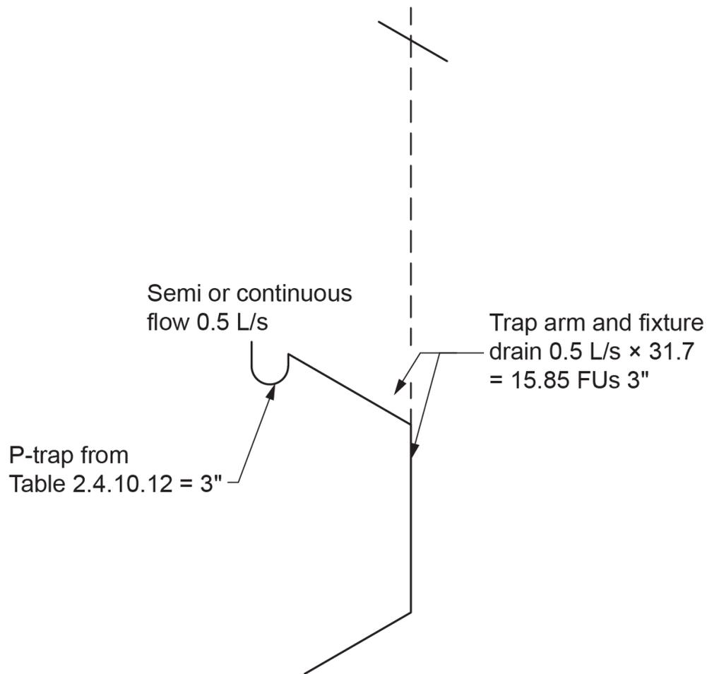
**Figure 2** Trap and fixture drain sizing based on semi or continuous flow. (Skilled Trades BC, 2021) Used with permission.
