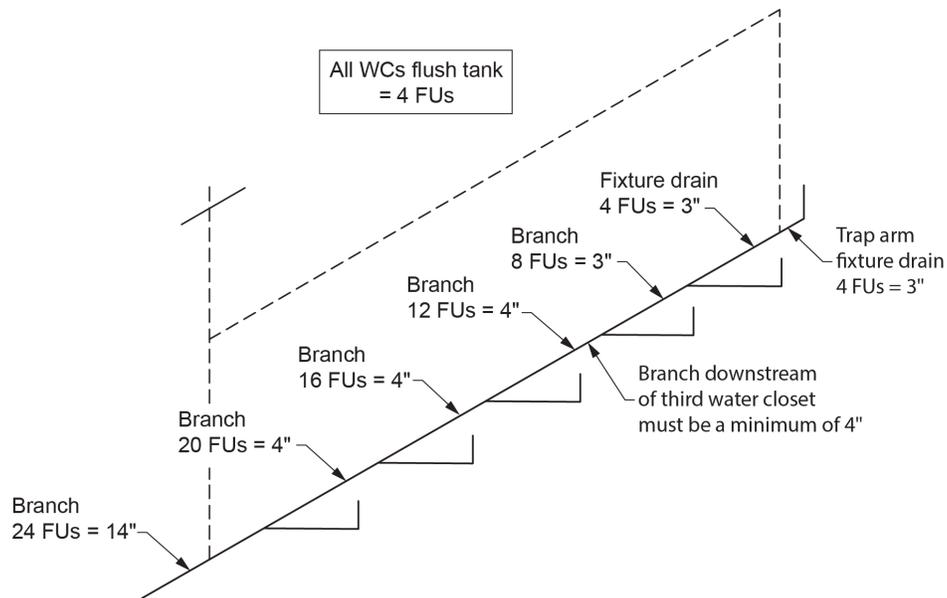
**Figure 5** Branch increasing to 4 in. in size due to the connection of a third water closet. (Skilled Trades BC, 2021) Used with permission.
