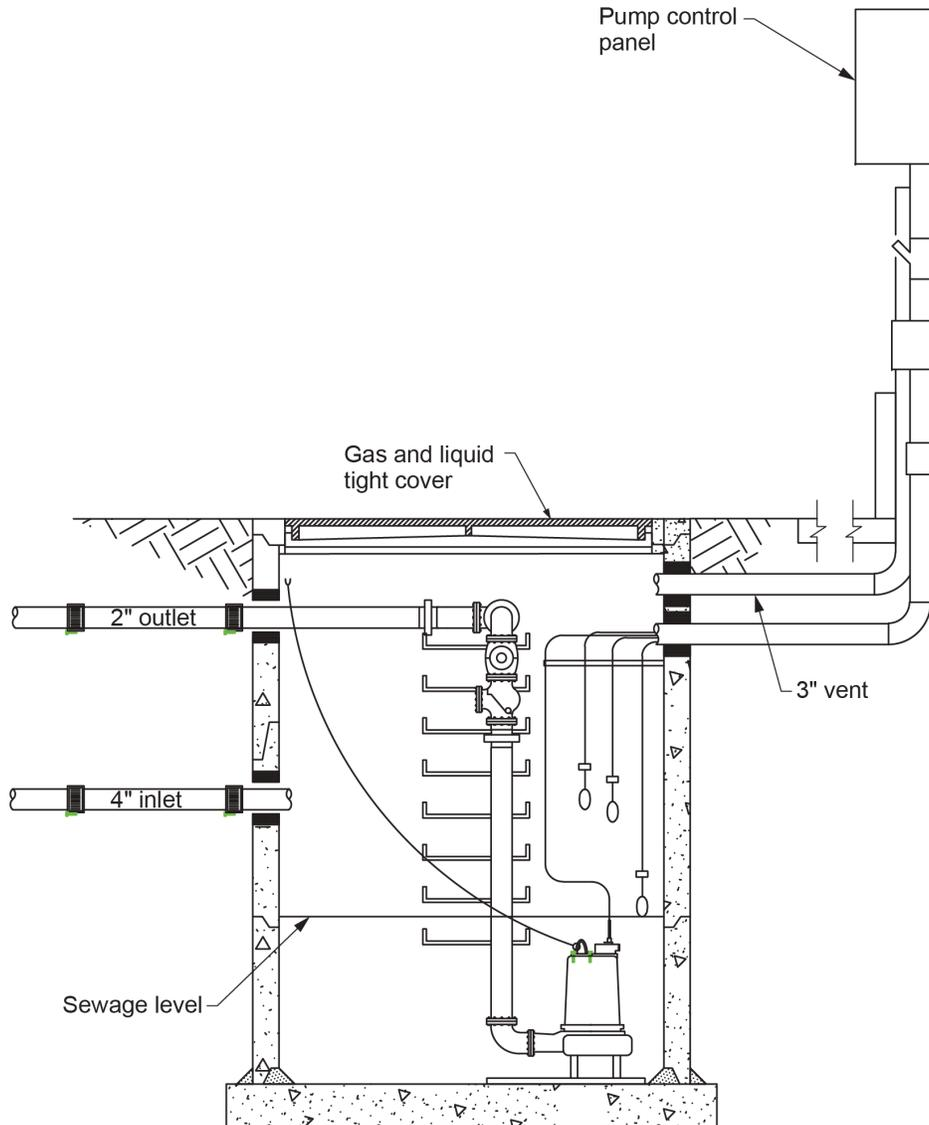
**Figure 8** Sewage sump basin with simplex pump. (Skilled Trades BC, 2021) Used with permission.
