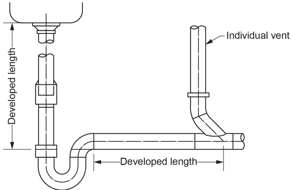
**Figure 12** Developed length of fixture outlet pipe and trap arm. (Skilled Trades BC, 2021) Used with permission.
