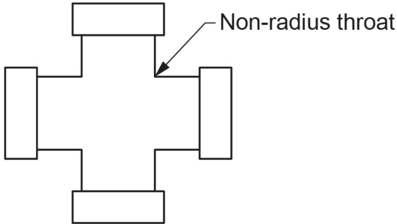
**Figure 3** Cross fitting is prohibited in a drainage system due to lack of throat radius. (Skilled Trades BC, 2021) Used with permission.
