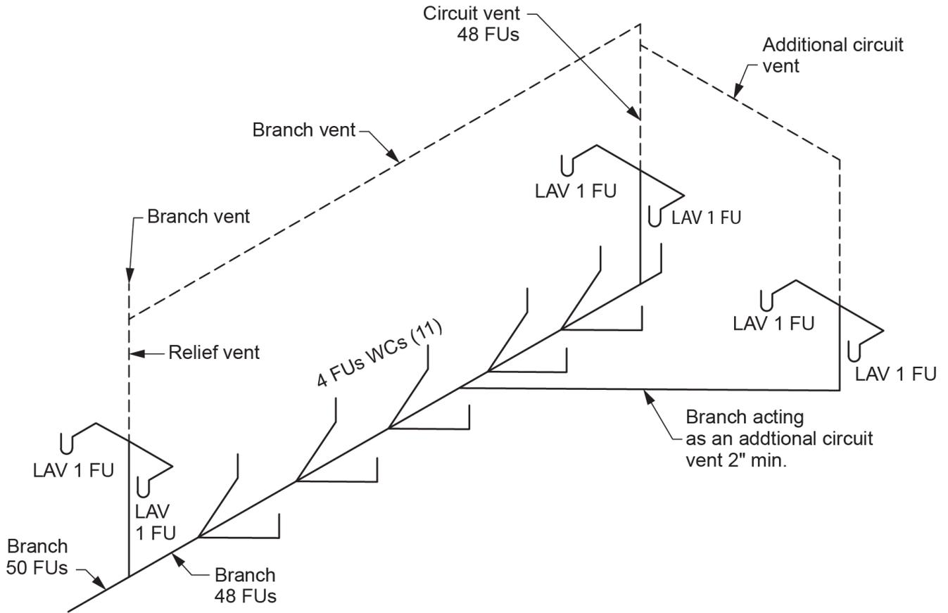
**Figure 24** The hydraulic load on a circuit vent is the connected load to the circuit-vented branch, including fixtures connected to the circuit vent and additional circuit vents. The load does not include the fixtures connected to the relief vent. (Skilled Trades BC, 2021) Used with permission.
