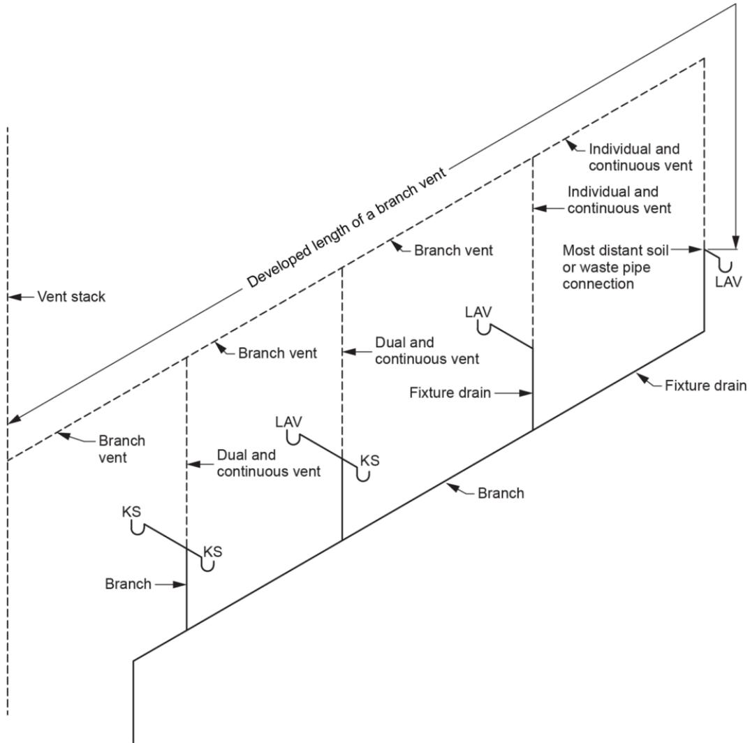
**Figure 1** Developed length of a branch vent. (Skilled Trades BC, 2021) Used with permission.
