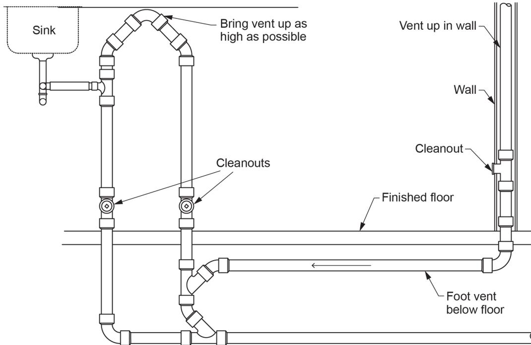
**Figure 18** Foot venting for island-vented sinks. (Skilled Trades BC, 2021) Used with permission.
