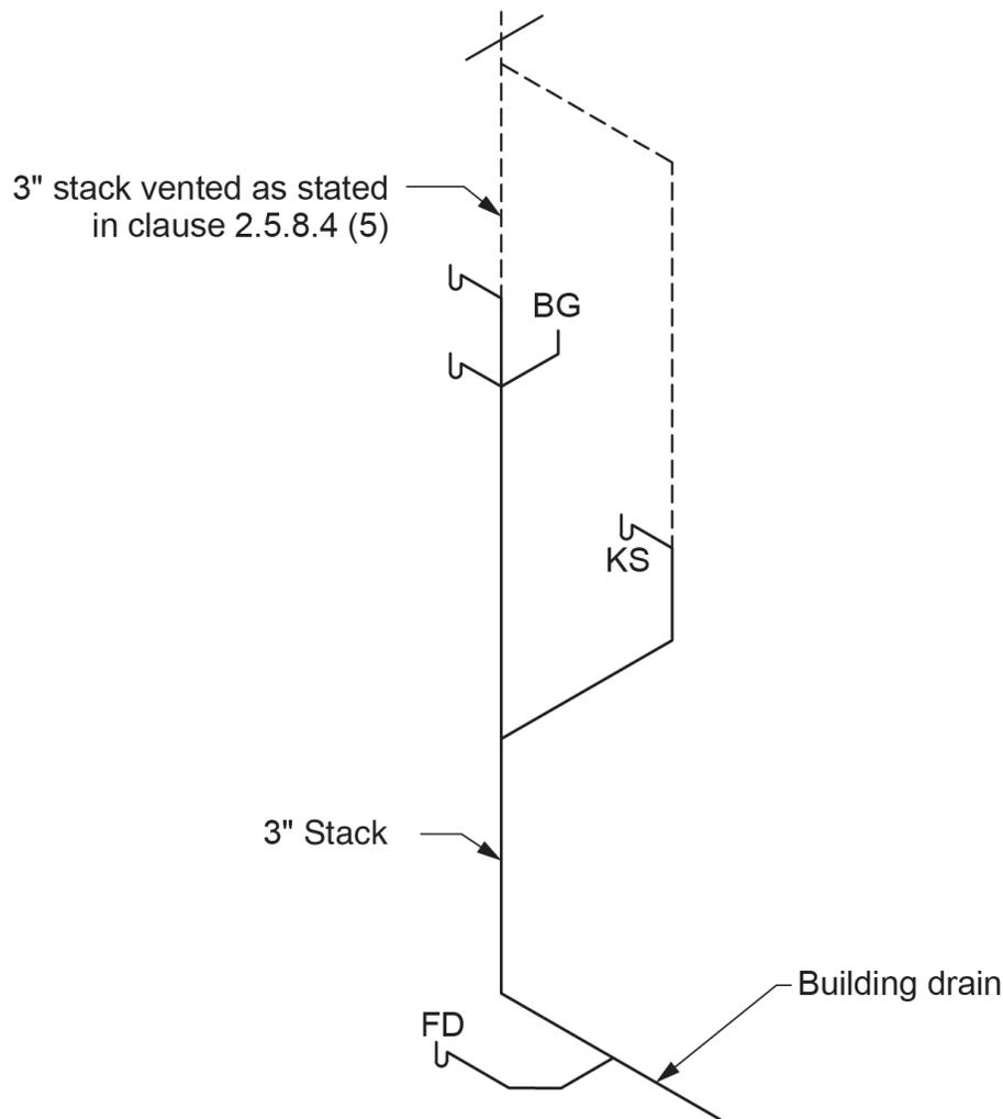
**Figure 2** Sizing of a stack vent in accordance with Clause 2.5.8.4.(5). (Skilled Trades BC, 2021) Used with permission.
