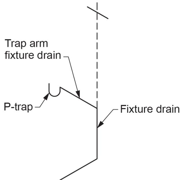
**Figure 3** Drainage pipe terminology serving a single fixture. (Skilled Trades BC, 2021) Used with permission.
