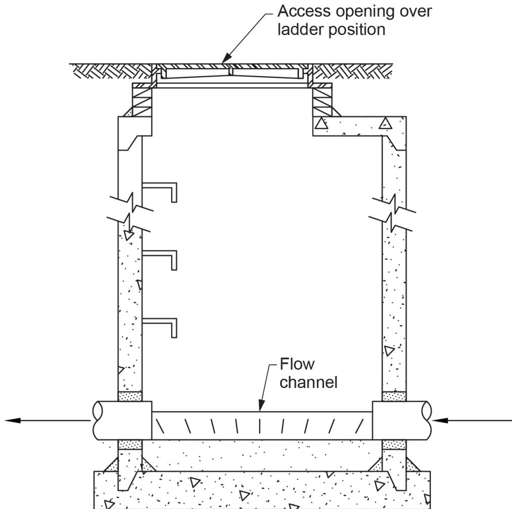
**Figure 9** Manhole used as a cleanout in large-diameter sanitary piping. (Skilled Trades BC, 2021) Used with permission.
