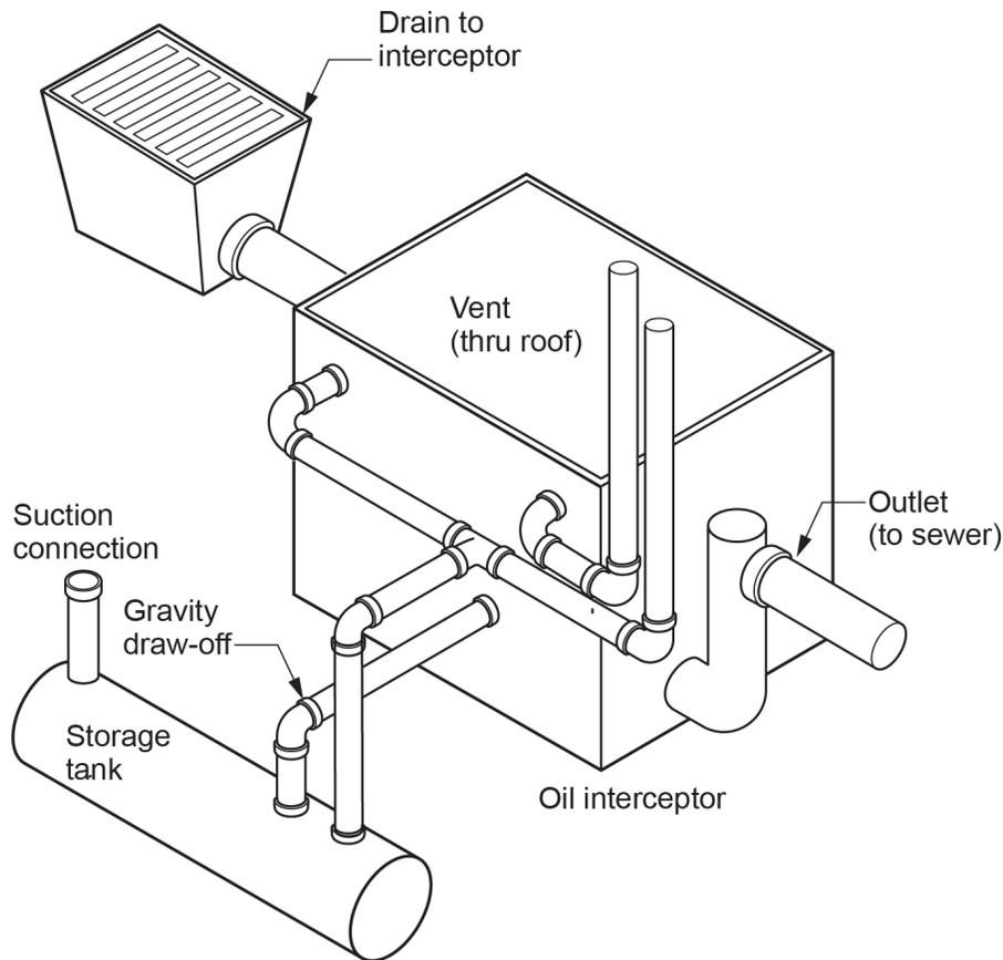
**Figure 7** Oil interceptor with separate storage tank. (Skilled Trades BC, 2021) Used with permission.
