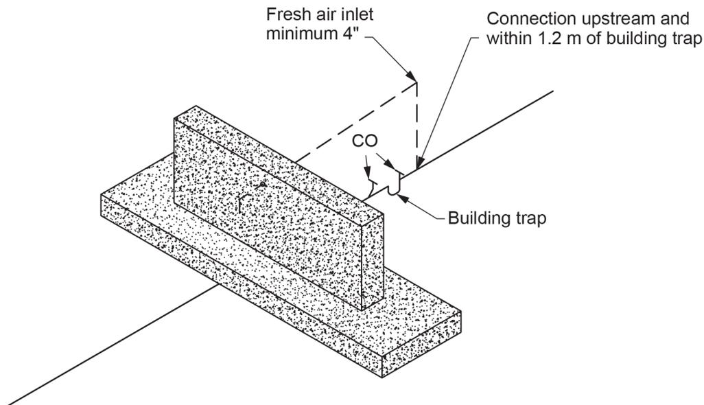
**Figure 19** NPC requirements for fresh air inlets. (Skilled Trades BC, 2021) Used with permission.
