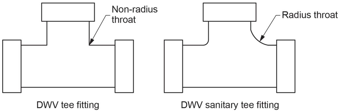
**Figure 1** The difference between a tee fitting and a sanitary tee fitting. (Skilled Trades BC, 2021) Used with permission.
