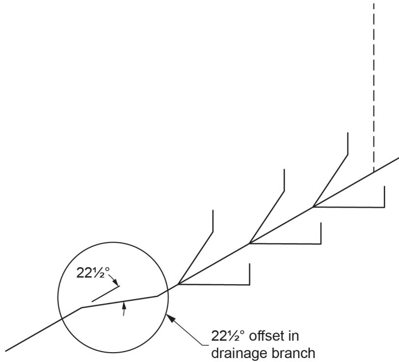
**Figure 22** Offset connecting two parallel drainage pipes. (Skilled Trades BC, 2021) Used with permission.
