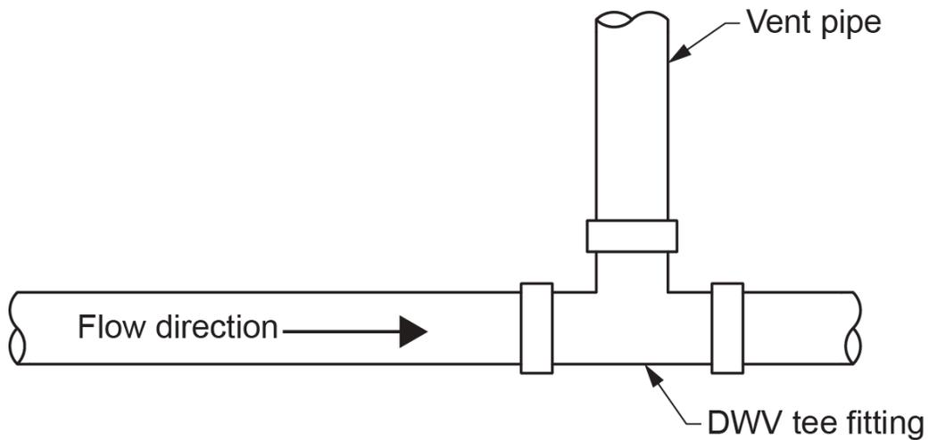
**Figure 2** Allowed installation for a DWV tee fitting. (Skilled Trades BC, 2021) Used with permission.
