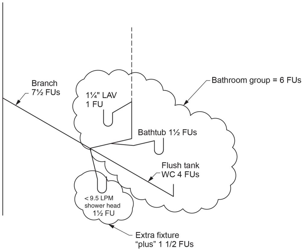
**Figure 8** Flush tank bathroom group with an additional single-headed shower. (Skilled Trades BC, 2021)
