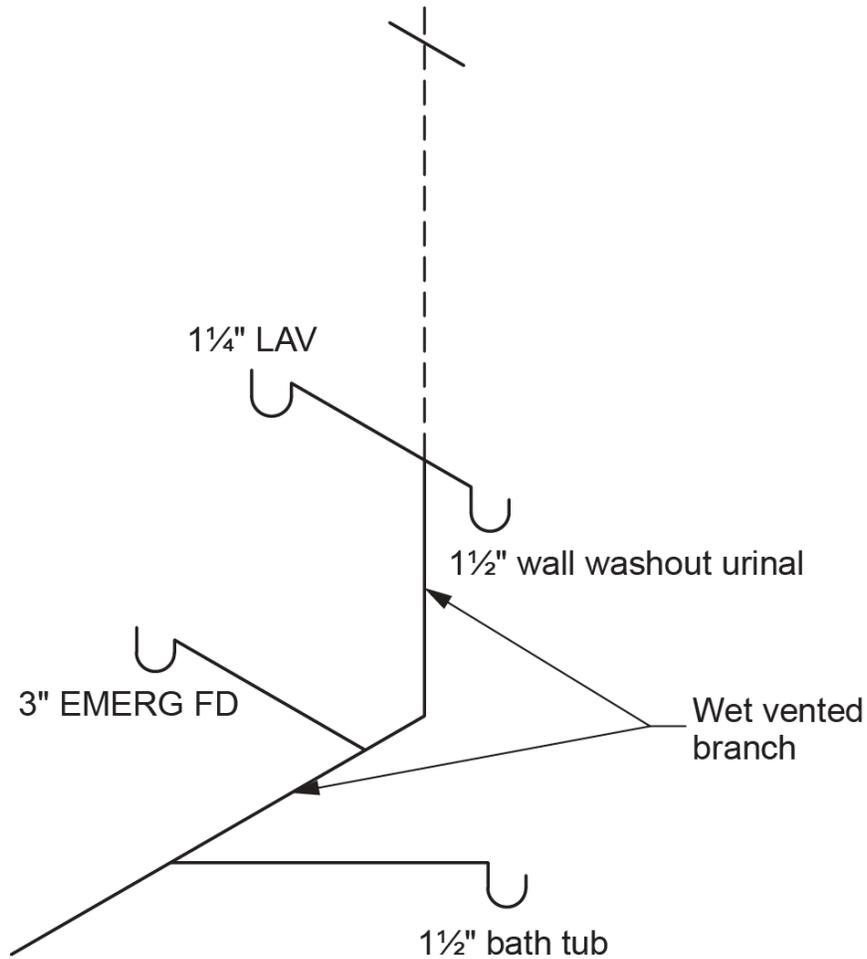
**Figure 4** A 3 in. emergency floor drain connected to a wet-vented branch. (Skilled Trades BC, 2021) Used with permission.
