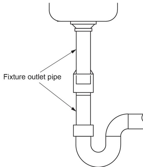
**Figure 15** Fixture outlet pipe. (Skilled Trades BC, 2021) Used with permission.
