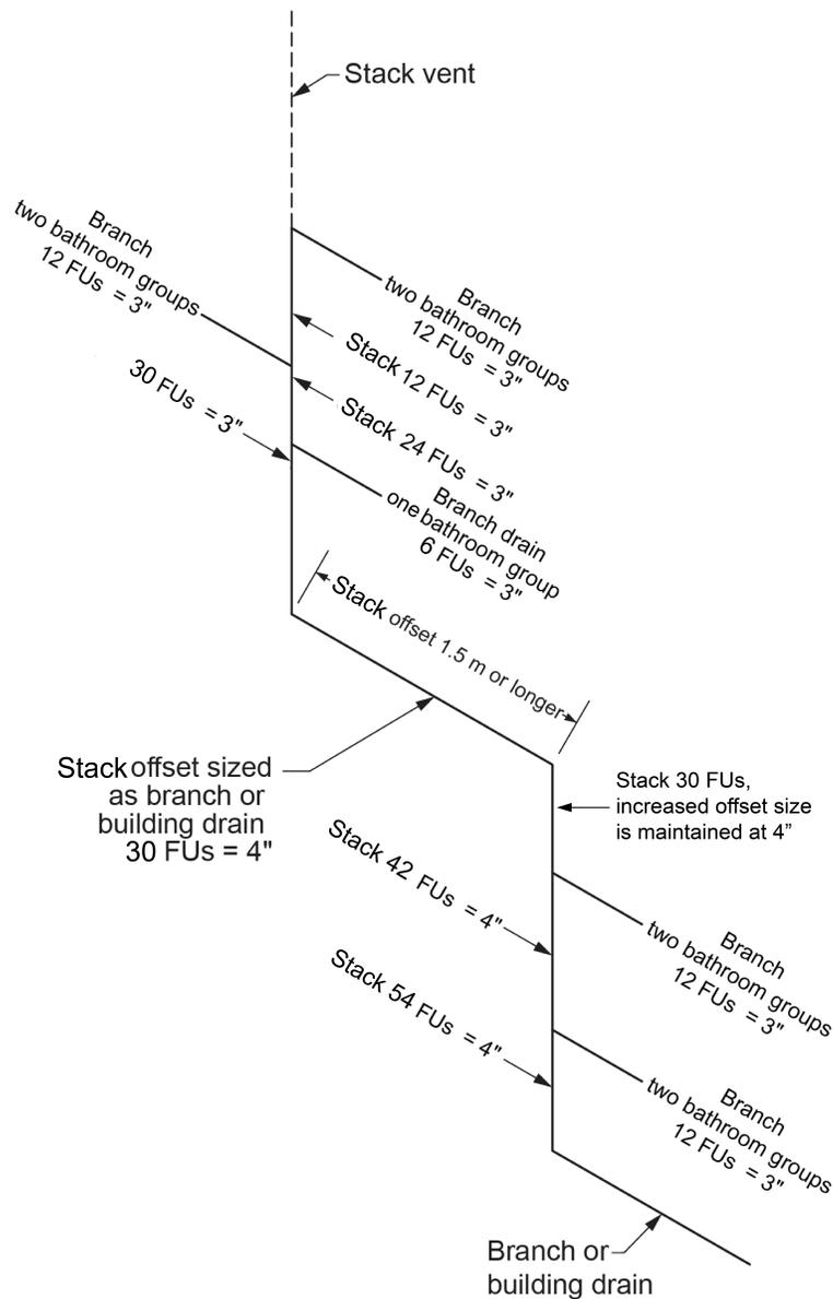
**Figure 9** Stack serving multiple bathroom groups with a nominally horizontal offset of 1.5 m or longer. (Skilled Trades BC, 2021) Used with permission.
