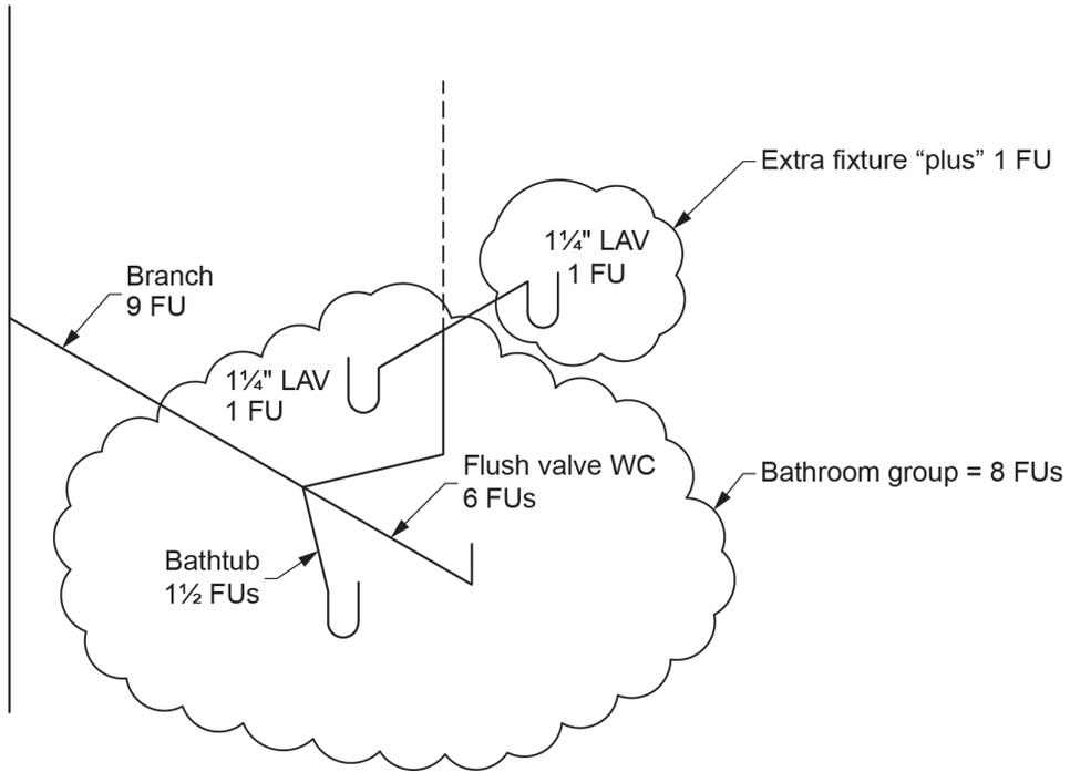
**Figure 7** Flush valve bathroom group with an additional lavatory basin. (Skilled Trades BC, 2021)
