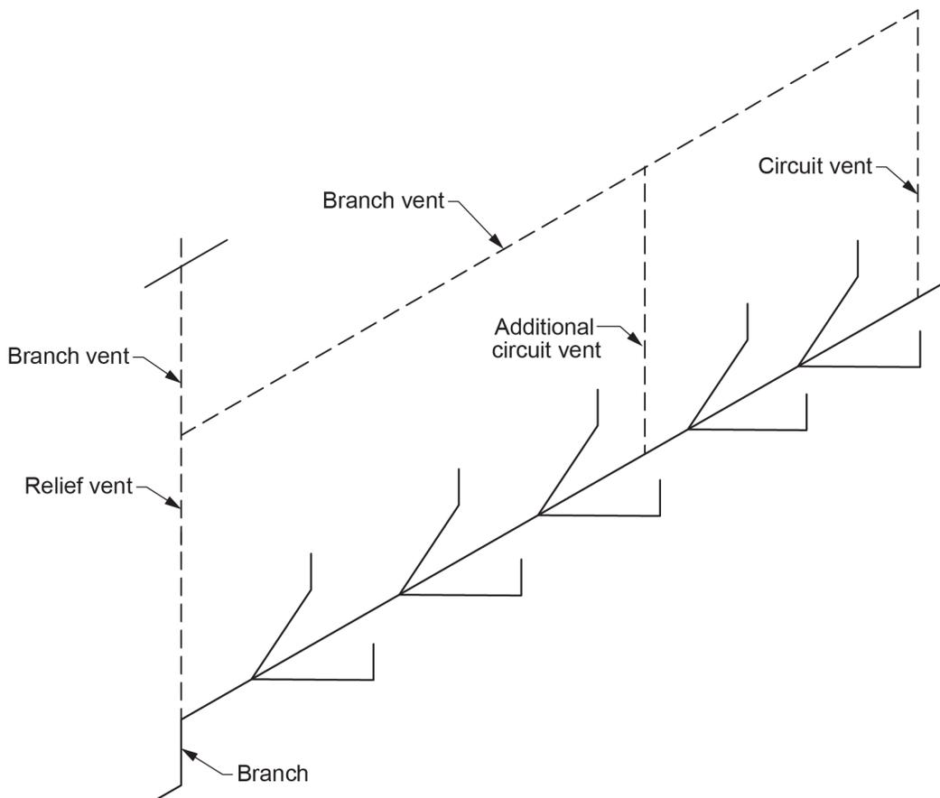
**Figure 1** Additional circuit vent. (Skilled Trades BC, 2021) Used with permission.
