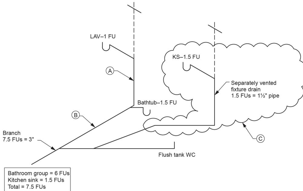
**Figure 7** The hydraulic load when a separately vented fixture is connected to the trap arm of a wet-vented water closet. (Skilled Trades BC, 2021) Used with permission.
