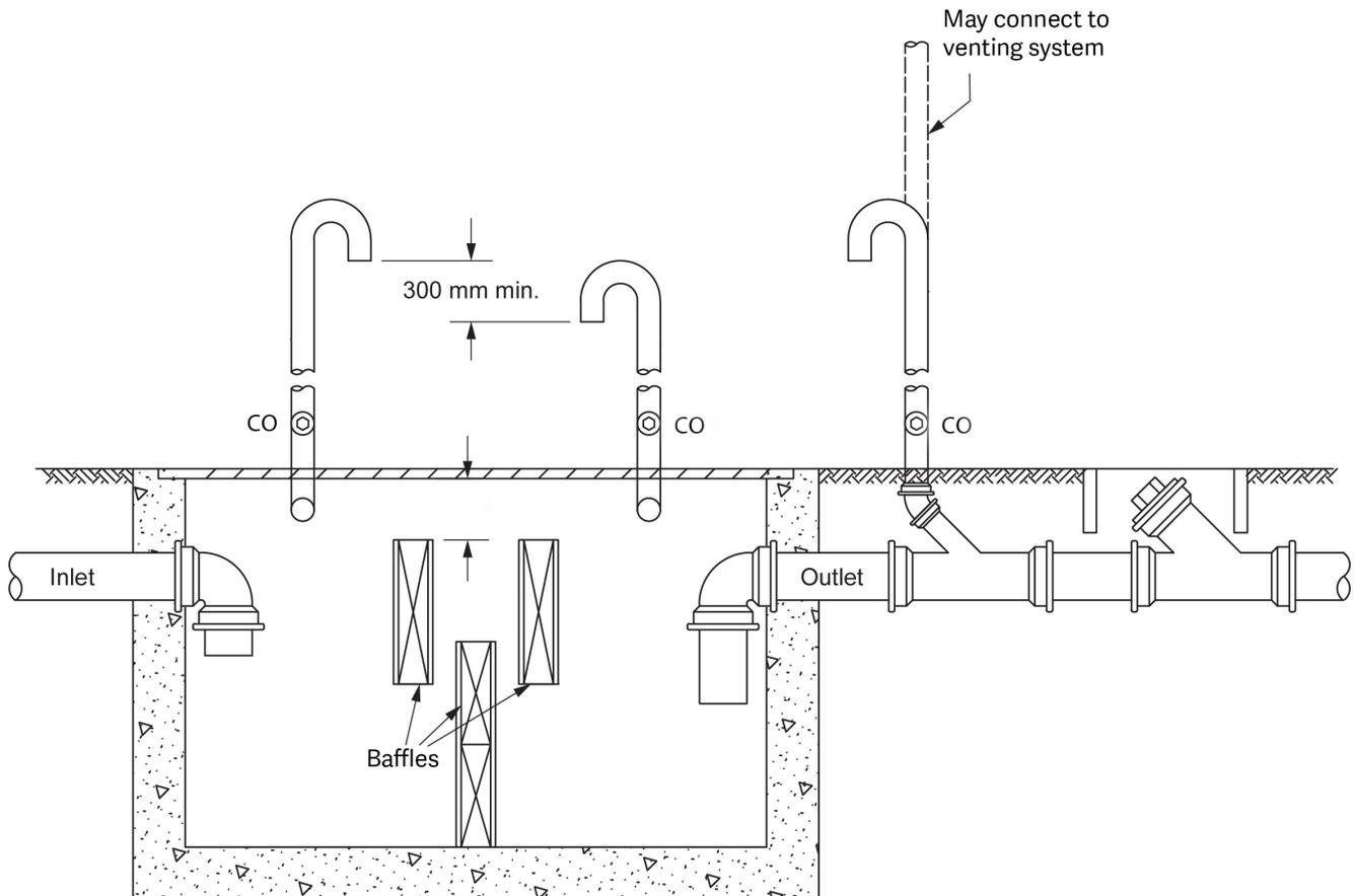
**Figure 20** NPC requirements for oil interceptor venting. (Skilled Trades BC, 2021) Used with permission.
