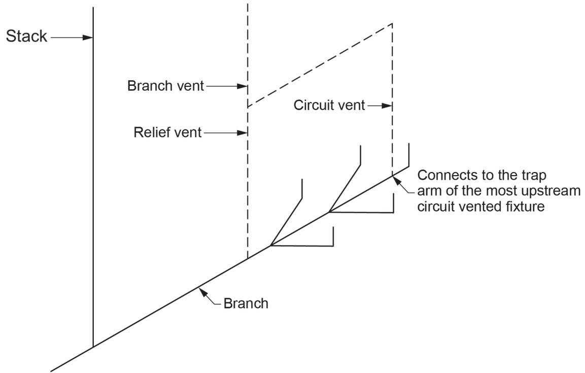
**Figure 4** Example of a circuit-vented branch. (Skilled Trades BC, 2021) Used with permission.
