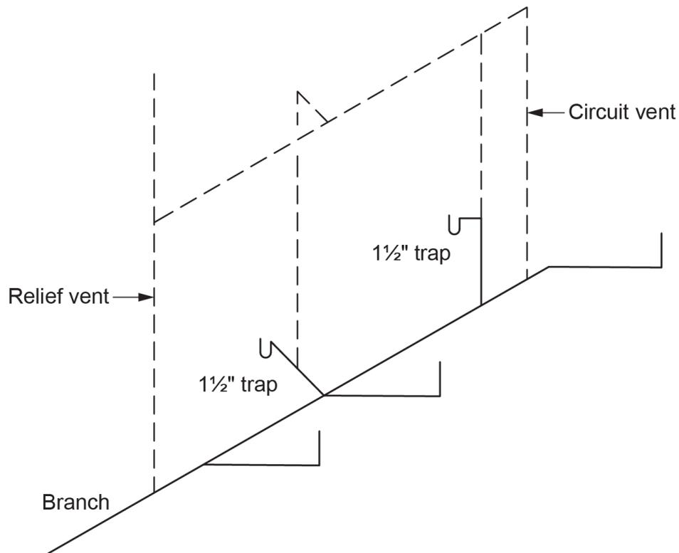
**Figure 5** Separately vented trap arm connected to a circuit-vented branch. (Skilled Trades BC, 2021) Used with permission.
