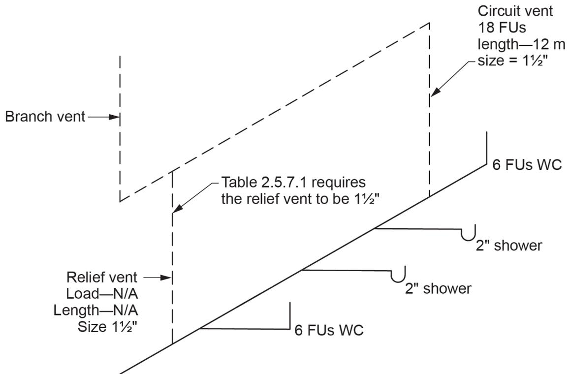
**Figure 21** Relief vent serving a circuit-vented branch. (Skilled Trades BC, 2021) Used with permission.
