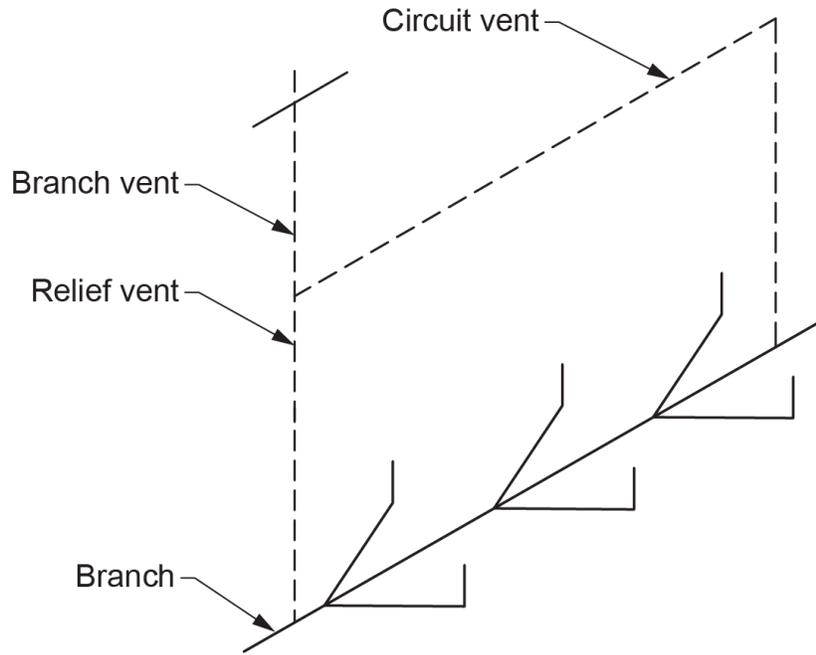
**Figure 15** Circuit vent serving a battery of WCs. (Skilled Trades BC, 2021) Used with permission.
