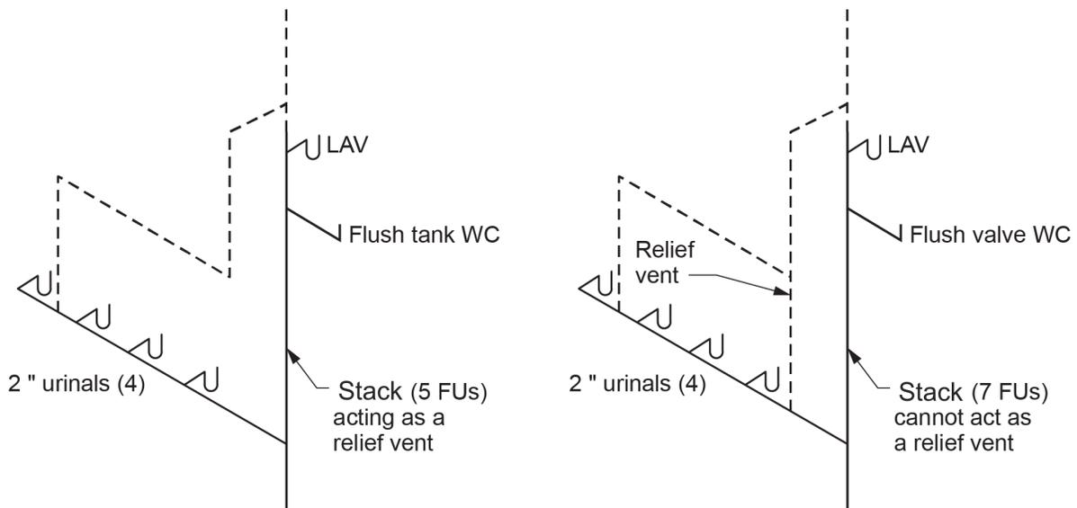
**Figure 10** Two examples of relief vents for a circuit-vented branch. (Skilled Trades BC, 2021) Used with permission.
