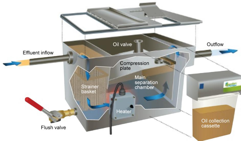
**Figure 3** Automatic grease interceptor (Image courtesy ACO, Inc.). All rights reserved.
