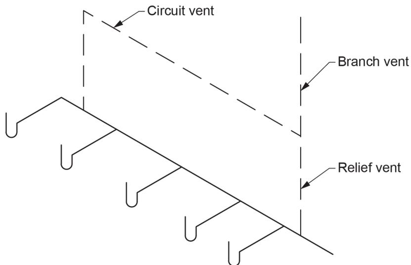
**Figure 16** Relief vent serving a circuit-vented branch. (Skilled Trades BC, 2021) Used with permission.
