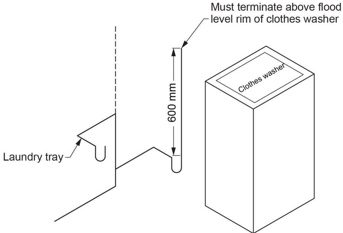
**Figure 8** NPC requirement for the installation of clothes washers. (Skilled Trades BC, 2021) Used with permission.
