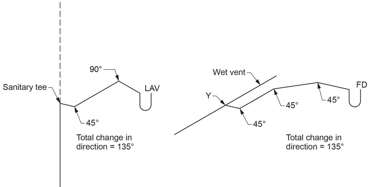
**Figure 14** NPC restriction on maximum change of direction of trap arms other than water closets. (Skilled Trades BC, 2021) Used with permission.
