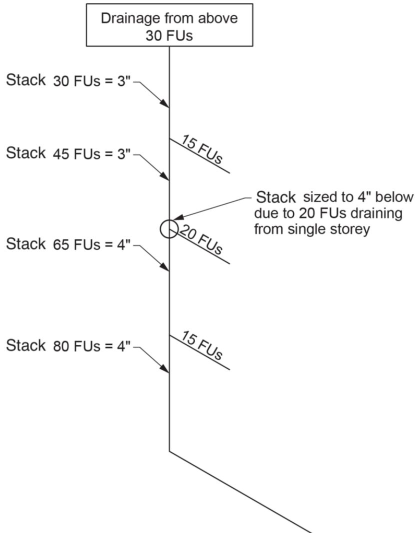
**Figure 4** Stack must be increased in size due to 20 FUs draining to it from any one storey. (Skilled Trades BC, 2021) Used with permission.
