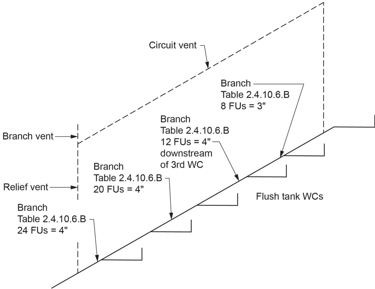
**Figure 16** Circuit-vented branch serving water closets sized as a branch from Table 2.4.10.6.-B. (Skilled Trades BC, 2021) Used with permission.
