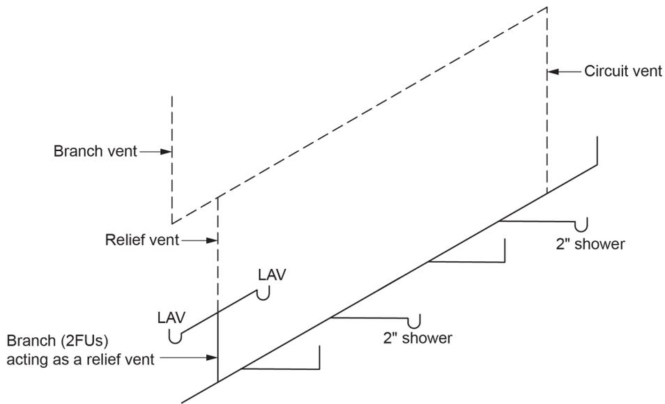
**Figure 8** A vertical branch acting as a relief vent for a circuit-vented branch. (Skilled Trades BC, 2021) Used with permission.
