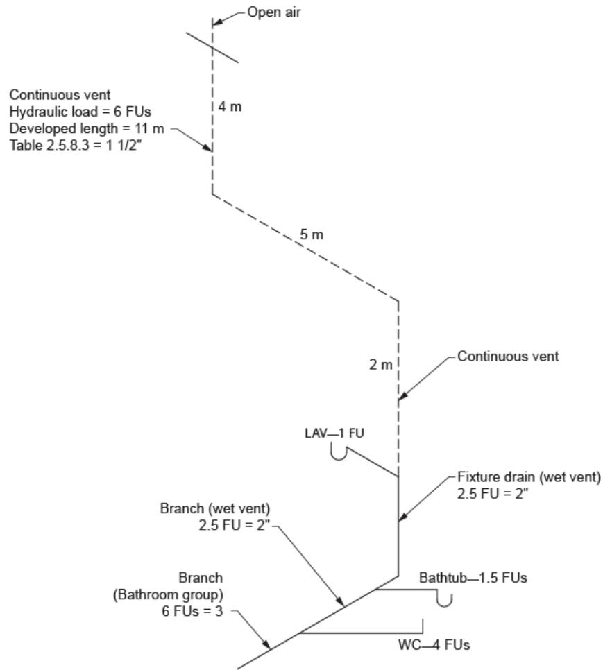
**Figure 11** Developed length and load of the vent. (Skilled Trades BC, 2021) Used with permission.
