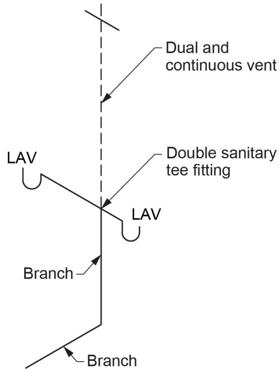
**Figure 14** Dual and continuous vent serving two lavatory basins. (Skilled Trades BC, 2021) Used with permission.
