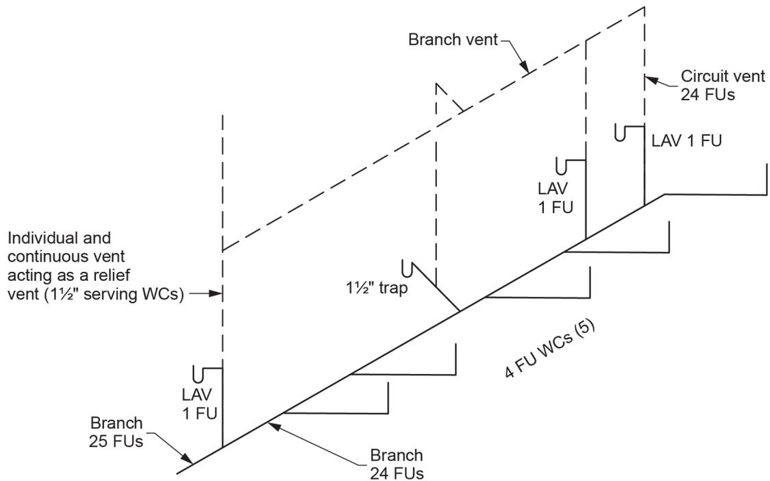
**Figure 25** The hydraulic load on a circuit vent is the connected load to the circuit-vented branch, including individually vented fixtures connected to the circuit vent. The load does not include the fixtures connected to the relief vent. (Skilled Trades BC, 2021) Used with permission.
