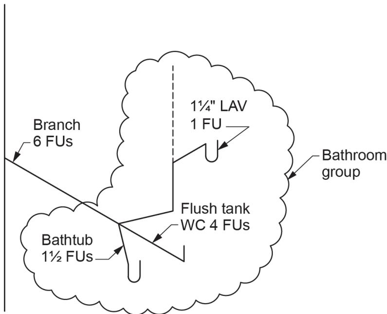
**Figure 6** Branch serving a bathroom group with a subsequent reduction in load on the system. (Skilled Trades BC, 2021) Used with permission.
