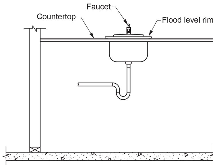
**Figure 16** Cabinet-mounted sink flood level rim. (Skilled Trades BC, 2021) Used with permission.
