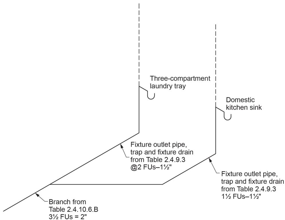
**Figure 3** Branch created by joining two fixture drains and sized from NPC Table 2.4.10.6.-B. (Skilled Trades BC, 2021) Used with permission.
