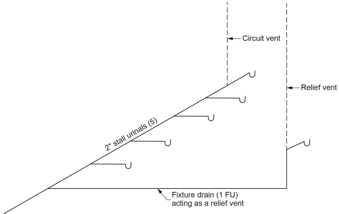
**Figure 9** A horizontal fixture drain acting as a relief vent for a circuit-vented branch. (Skilled Trades BC, 2021) Used with permission.
