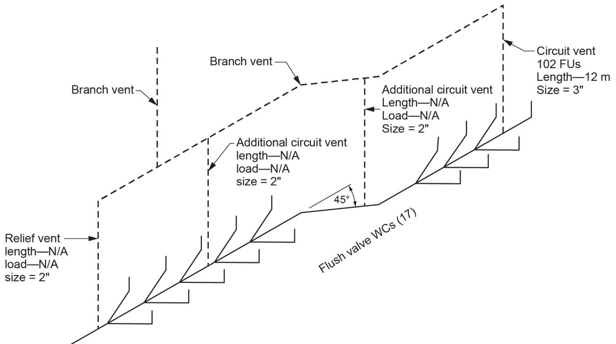
**Figure 20** Relief vent and additional circuit vents serving a circuit-vented branch. (Skilled Trades BC, 2021) Used with permission.
