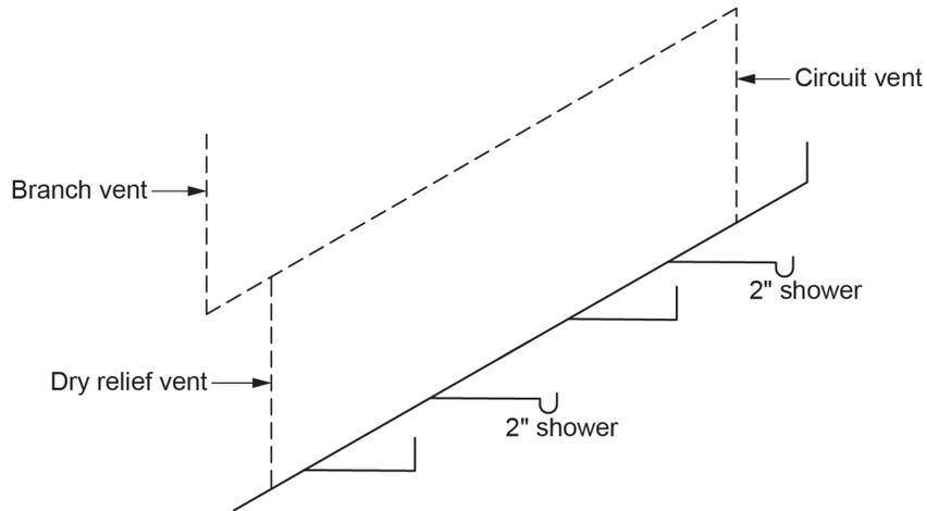
**Figure 7** A dry vent acting as a relief vent for a circuit-vented branch. (Skilled Trades BC, 2021) Used with permission.
