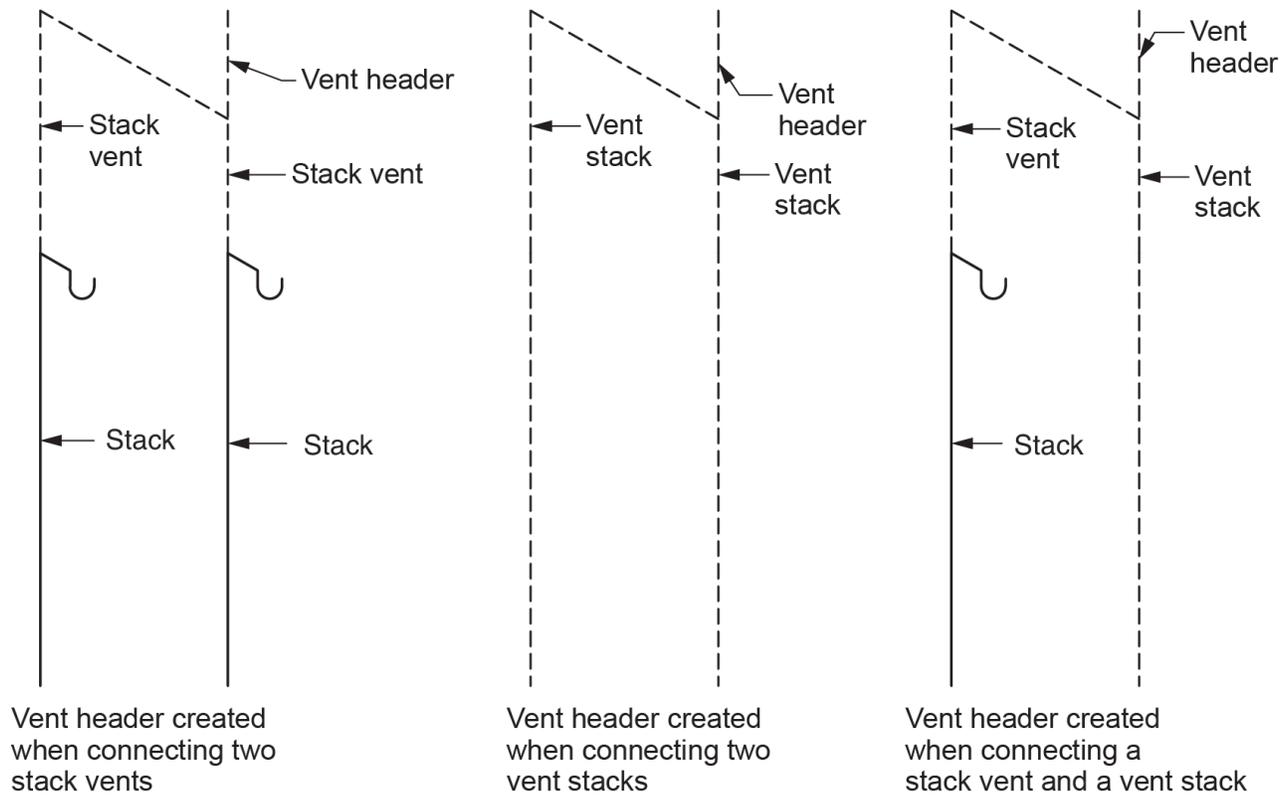
**Figure 21** Vent header combinations. (Skilled Trades BC, 2021) Used with permission.
