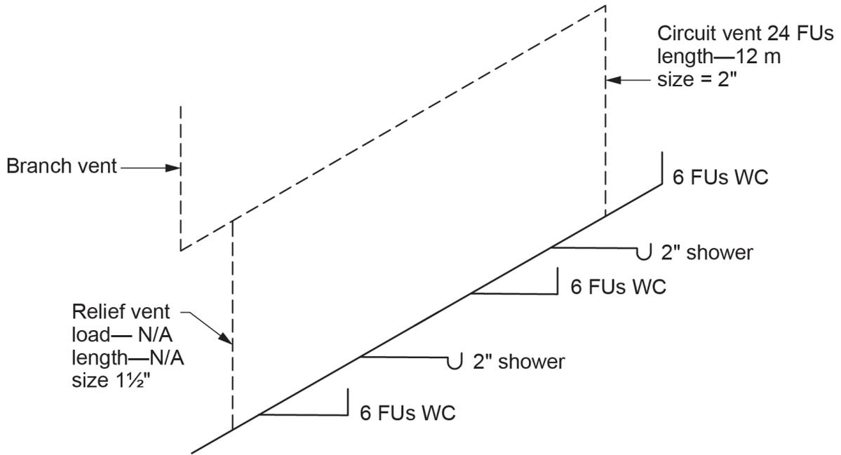
**Figure 19** Relief vent serving a circuit-vented branch one size smaller than circuit vent and in compliance with Table 2.5.7.1. (Skilled Trades BC, 2021) Used with permission.
