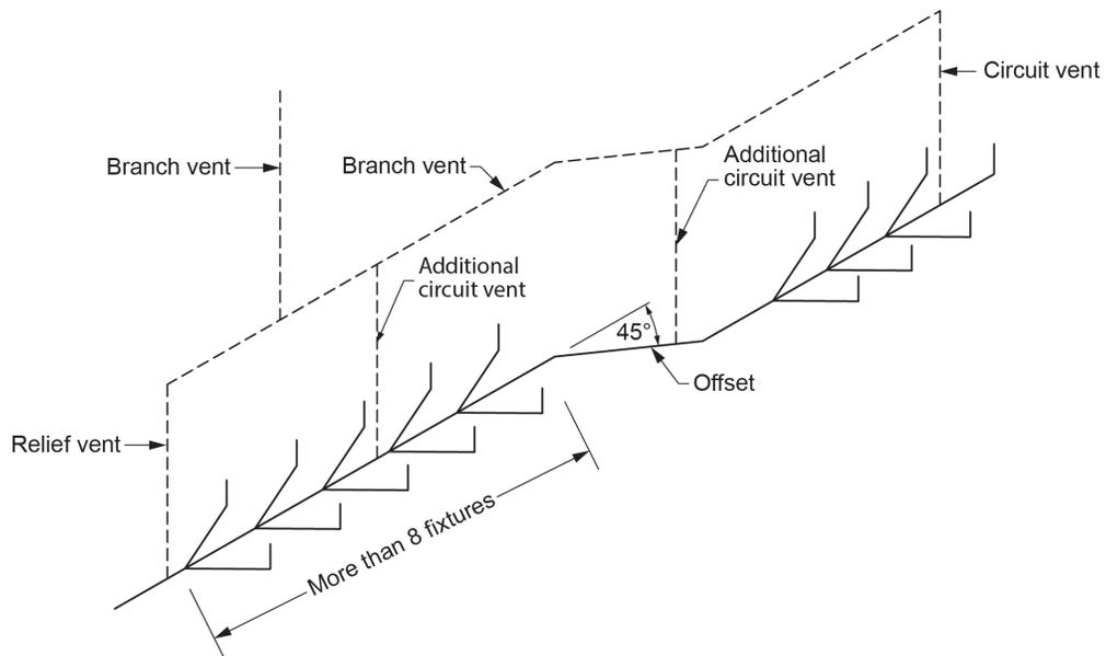
**Figure 12** Additional circuit vents added to meet Clause 2.5.3.1, with labeled branch vents, additional circuit vents, relief vent, and more than 5 fixtures connected with a 45-degree offset. (Skilled Trades BC, 2021) Used with permission.
