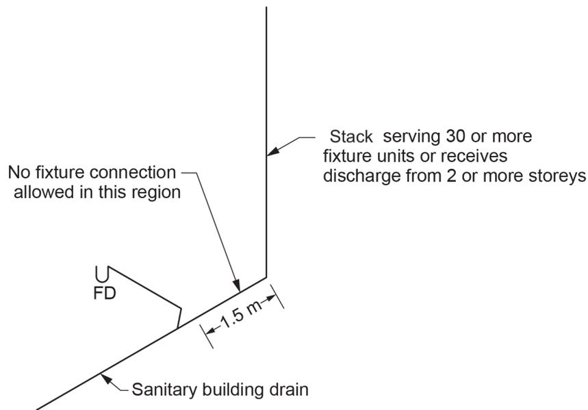
**Figure 10** NPC restrictions when connecting to a nominally horizontal sanitary drainage pipe serving a stack. (Skilled Trades BC, 2021) Used with permission.
