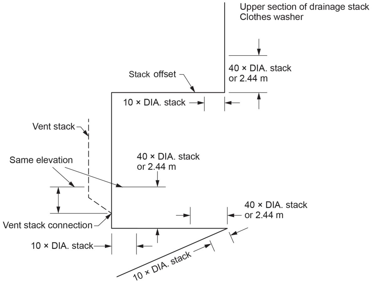
**Figure 11** NPC restrictions when connecting to a sanitary drainage pipe that serves two or more clothes washers. (Skilled Trades BC, 2021) Used with permission.
