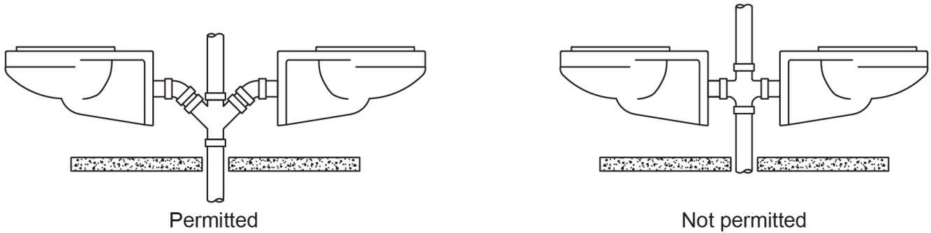
**Figure 5** NPC restrictions for double sanitary tee fittings serving back-to-back back outlet water closets. (Skilled Trades BC, 2021) Used with permission.
