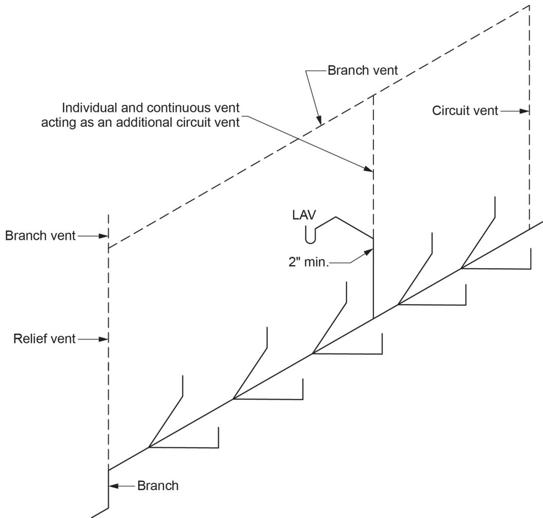
**Figure 13** Sanitary drainage pipe acting as an additional circuit vent. (Skilled Trades BC, 2021) Used with permission.
