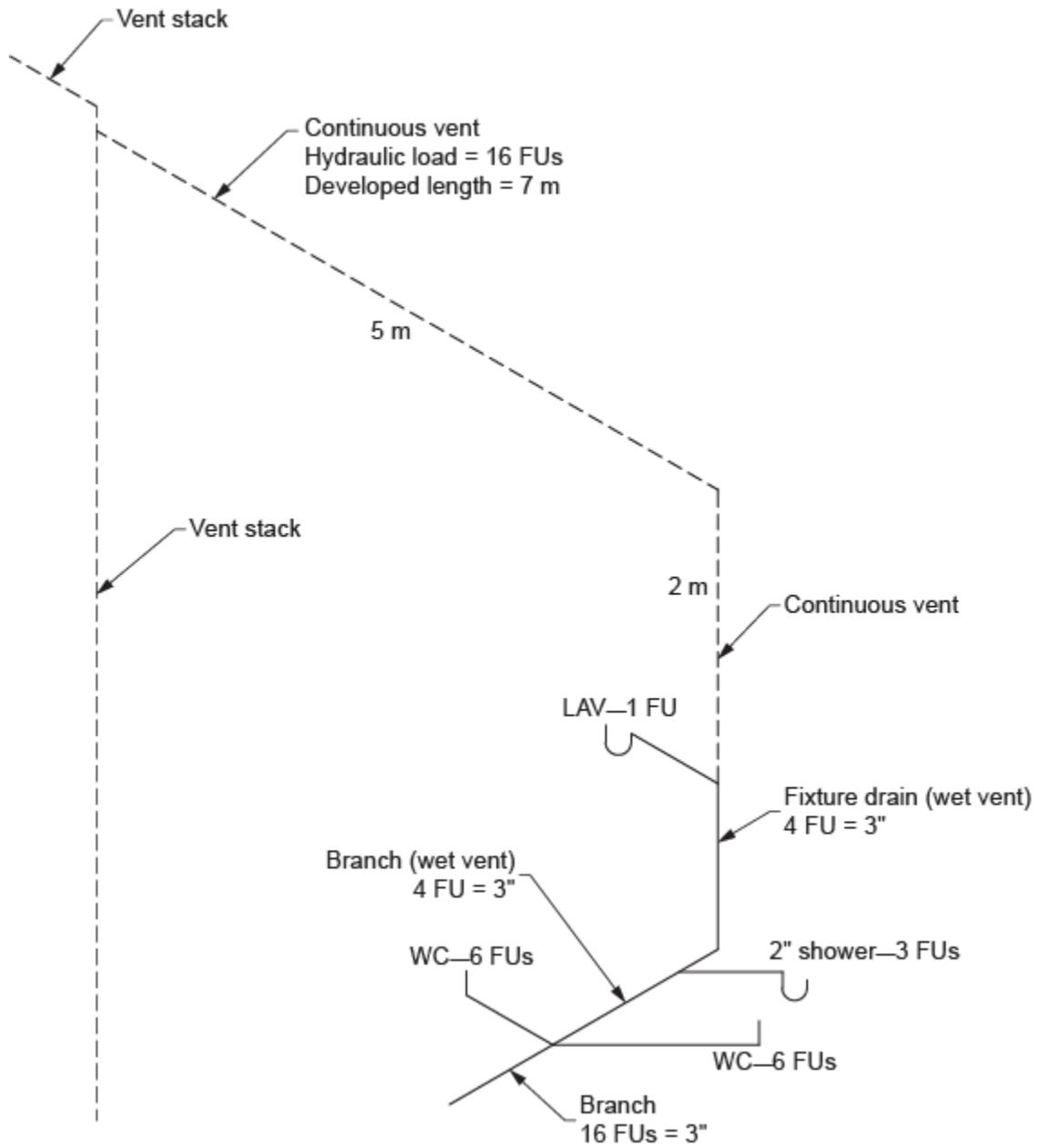
**Figure 12** Continuous vent sizing overridden by Table 2.5.7.1. (Skilled Trades BC, 2021) Used with permission.
