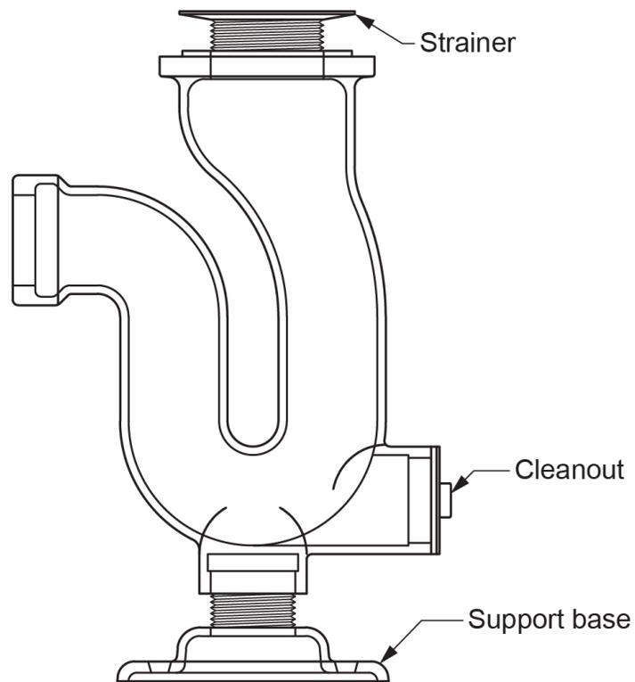
**Figure 28** P-trap standard. (Skilled Trades BC, 2021) Used with permission.
