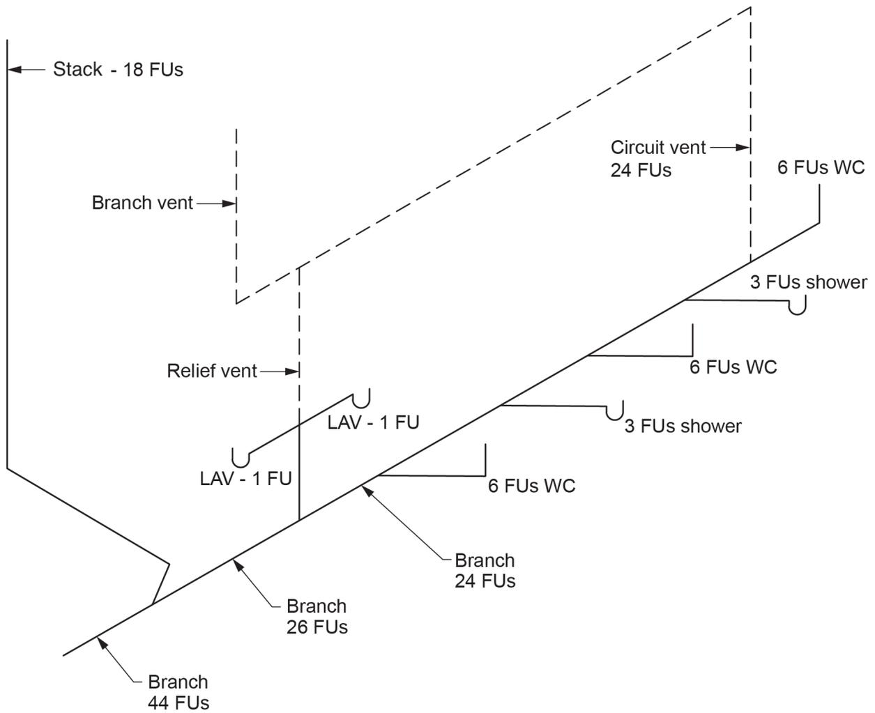
**Figure 22** The hydraulic load on a circuit vent is the connected load to the circuit-vented branch, not including the fixtures connected to the relief vent. (Skilled Trades BC, 2021) Used with permission.
