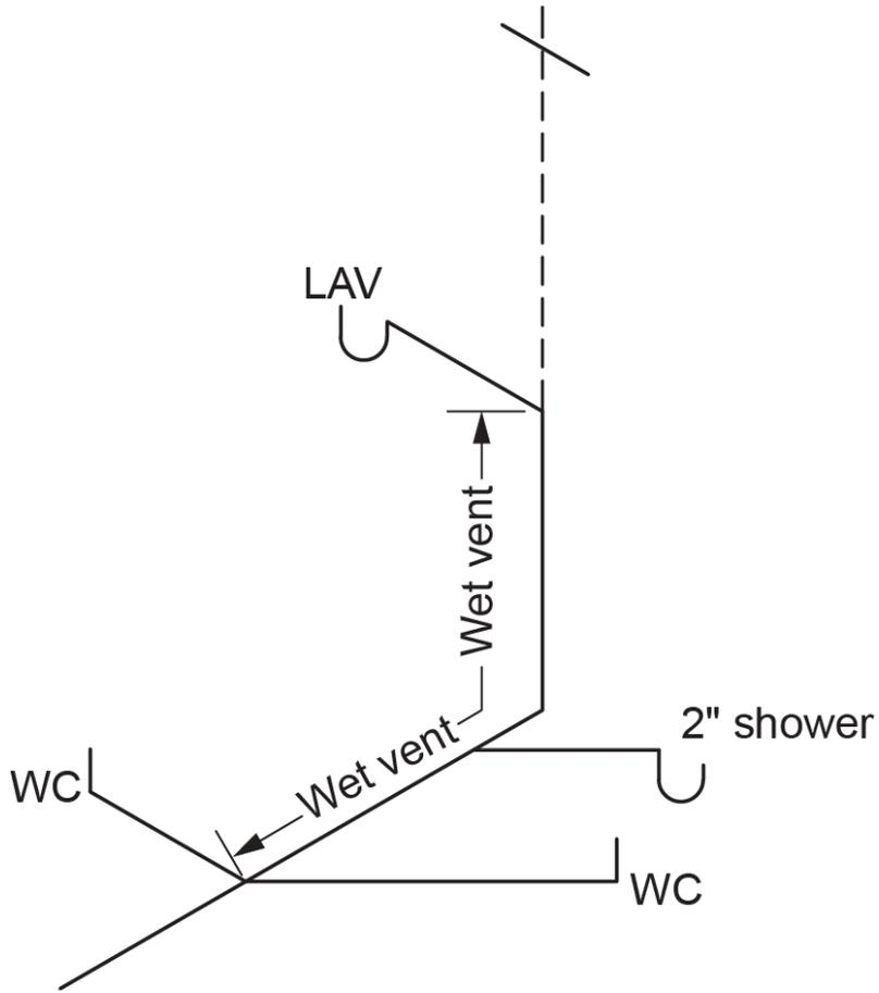
**Figure 3** Maximum of two water closets connected to a wet vent. (Skilled Trades BC, 2021) Used with permission.
