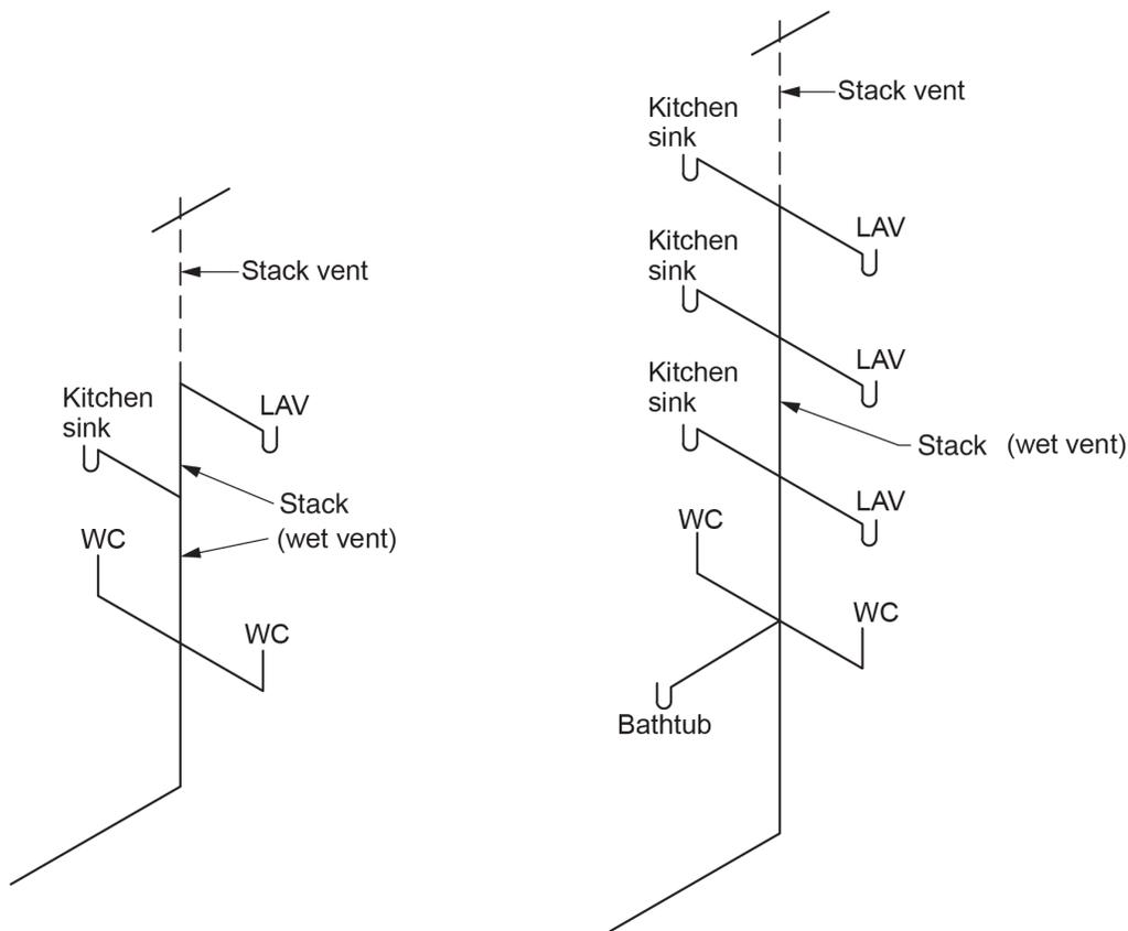
**Figure 1** Water closets connected to a multi-storey wet vent. (Skilled Trades BC, 2021) Used with permission.
