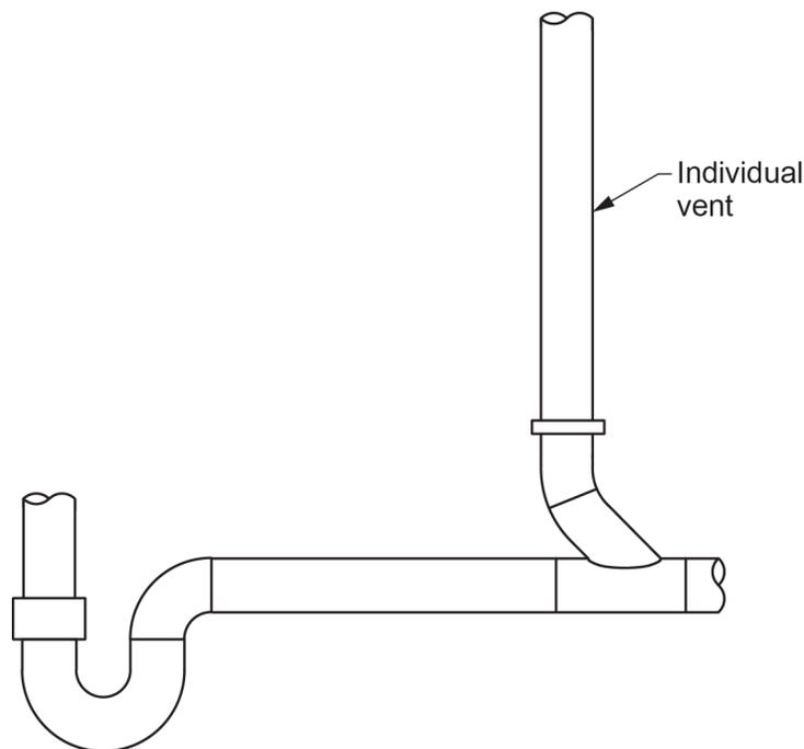
**Figure 10** Individual vent serving a fixture connected to the horizontal trap arm. (Skilled Trades BC, 2021) Used with permission.
