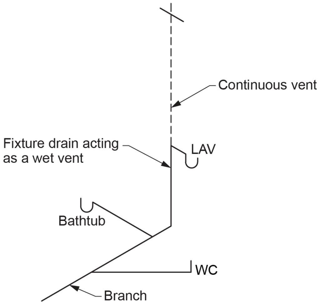
**Figure 12** Continuous vent serving a wet-vented bathroom group. (Skilled Trades BC, 2021) Used with permission.
