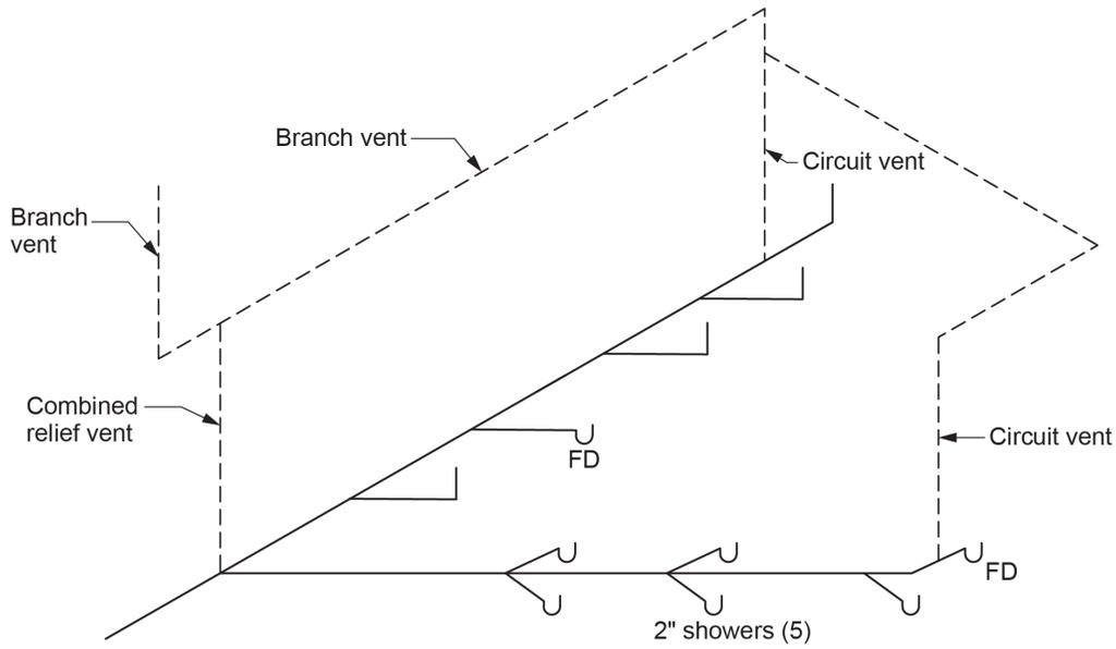
**Figure 11** A symmetrical connection used to join a combined relief vent when serving two circuit-vented branches. (Skilled Trades BC, 2021) Used with permission.
