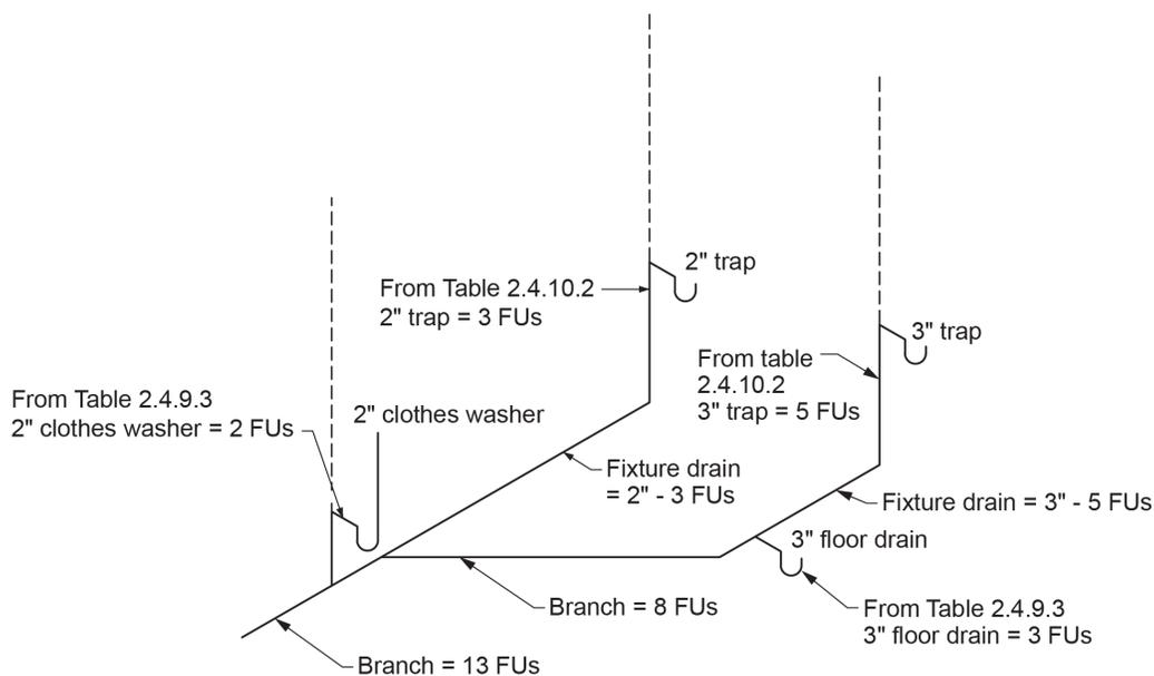
**Figure 1** Drainage system showing different fixture unit ratings for unknown traps and fixture designations. (Skilled Trades BC, 2021) Used with permission.
