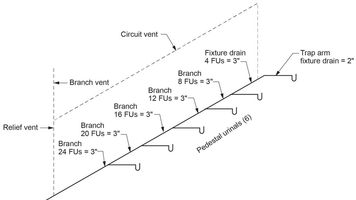
**Figure 18** Circuit-vented branch serving 2 in. urinals increased to 3 in. fixture drain downstream of the circuit vent connection. (Skilled Trades BC, 2021) Used with permission.
