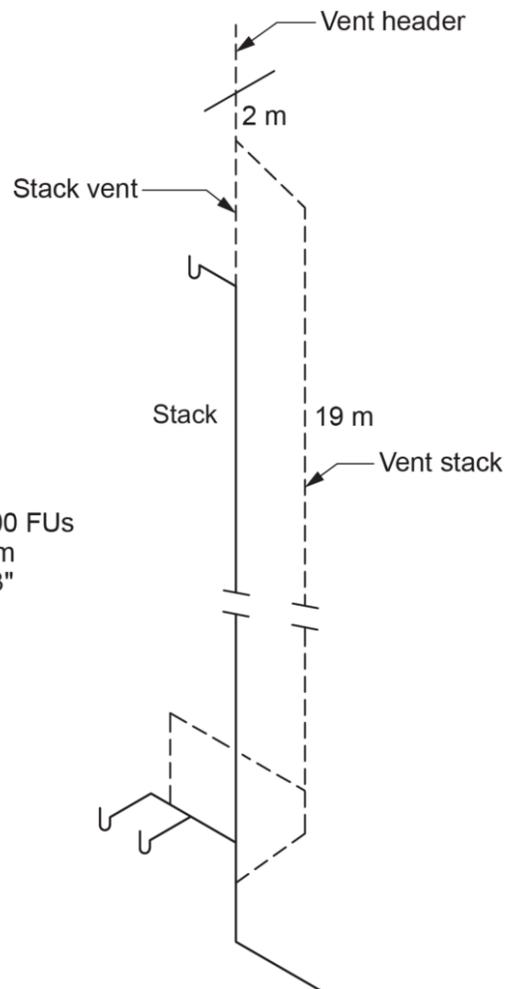
**Figure 3** Sizing of a vent stack using Table 2.5.8.4. (Skilled Trades BC, 2021) Used with permission.
