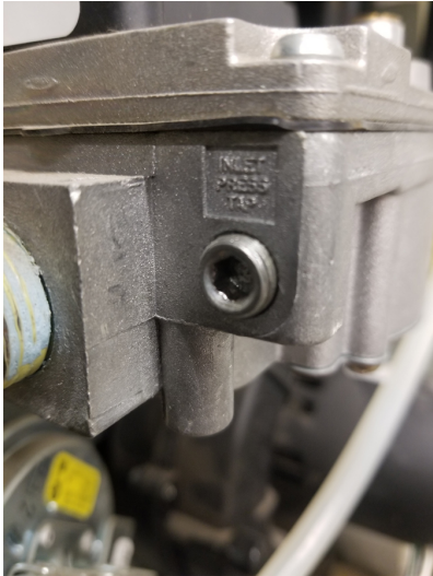
Figure 15 \frac{1}{8} in. (0.125 in.) NPT inlet pressure tap plug (left), outlet pressure tap connected to clear plastic manometer tubing (right). (Rod Lidstone) CC BY ( https://creativecommons.org/licenses/by/4.0/ )
