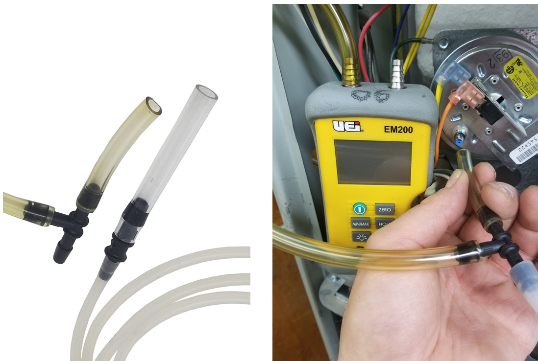
Figure 18 Barbed reducer and barbed tee (left), manometer being connected into pressure switch sensing line (right). (Rod Lidstone) CC BY ( https://creativecommons.org/licenses/by/4.0/ )
