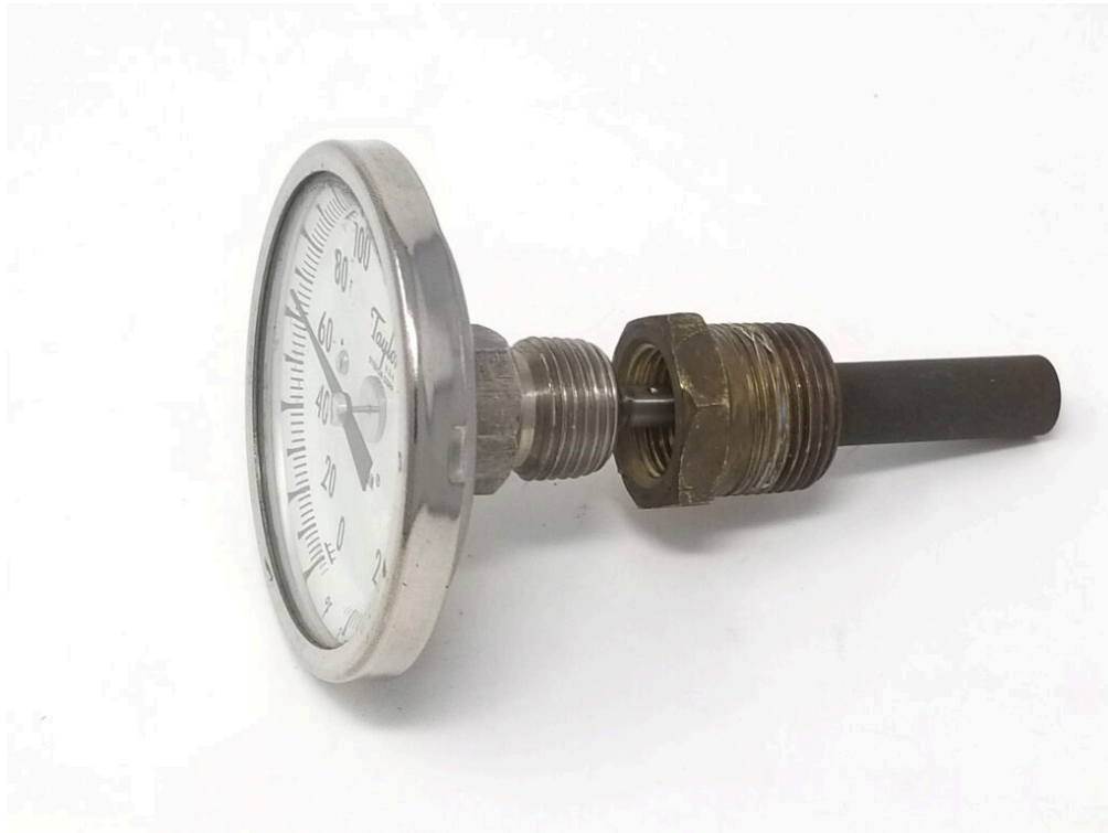
Figure 4 Dial thermometer partially inserted into thermowell. (Rod Lidstone) CC BY ( https://creativecommons.org/licenses/by/4.0/ )
