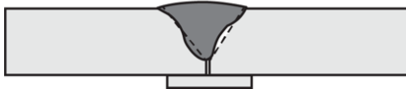
Figure 7 Lack of fusion (BC Industry Training Authority, 2019). CC BY-NC-SA 4.0 ( https://creativecommons.org/licenses/by-nc-sa/4.0/ )
