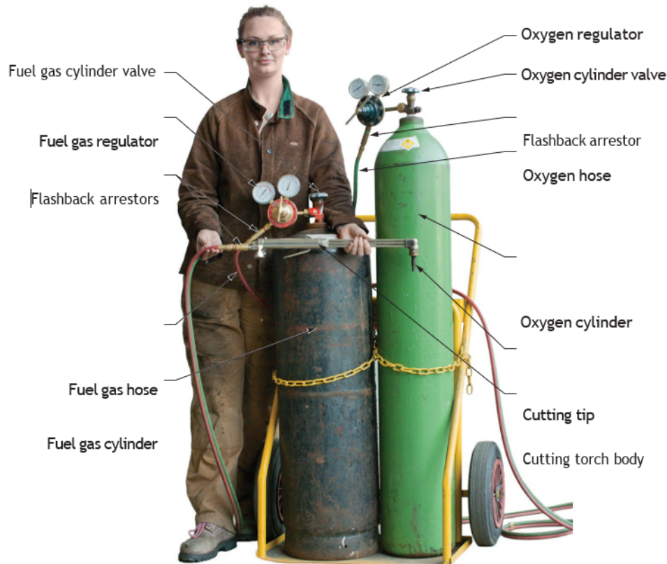
Figure 1 Portable oxy-acetylene setup (BC Industry Training Authority, 2019). CC BY-NC-SA 4.0 ( https://creativecommons.org/licenses/by-nc-sa/4.0/ )
