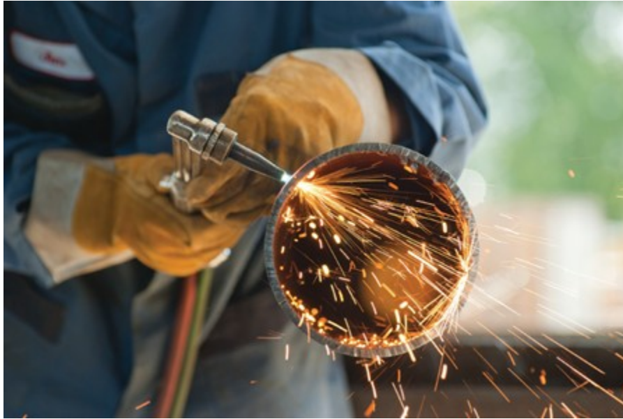
Figure 2 Oxy-fuel gas cutting process (BC Industry Training Authority, 2019). CC BY-NC-SA 4.0 ( https://creativecommons.org/licenses/by-nc-sa/4.0/ )
