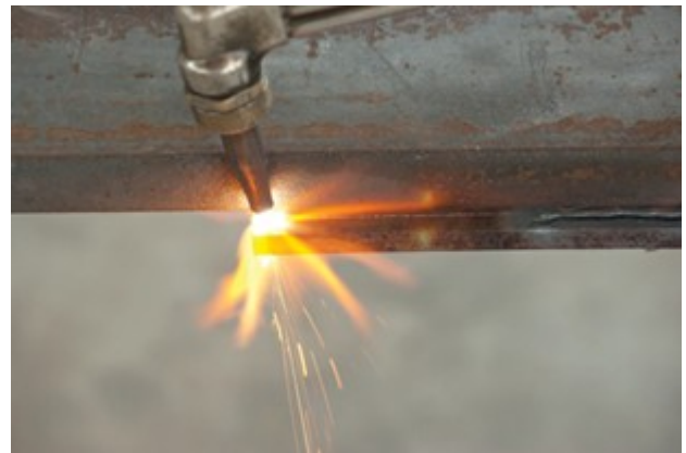
Figure 6 One method of starting the cut (BC Industry Training Authority, 2019). CC BY-NC-SA 4.0 ( https://creativecommons.org/licenses/by-nc-sa/4.0/ )
