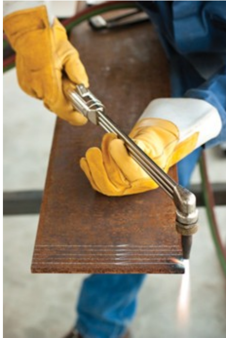
Figure 4 One hand guides the torch, the other acts as a pivot (BC Industry Training Authority, 2019). CC BY-NC-SA 4.0 ( https://creativecommons.org/licenses/by-nc-sa/4.0/ )
