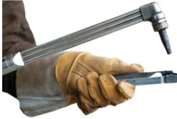
Figure 4 Correct striker position (BC Industry Training Authority, 2019). CC BY-NC-SA 4.0 ( https://creativecommons.org/licenses/by-nc-sa/4.0/ )
