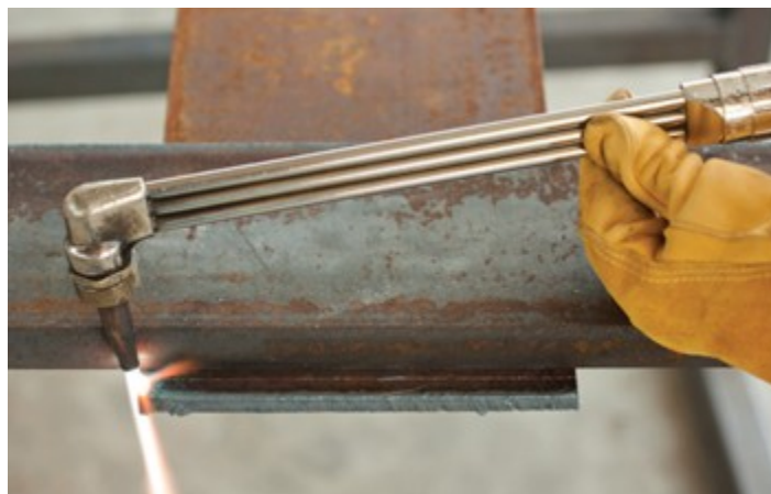
Figure 5 Technique for starting a straight cut (BC Industry Training Authority, 2019). CC BY-NC-SA 4.0 ( https://creativecommons.org/licenses/by-nc-sa/4.0/ )
