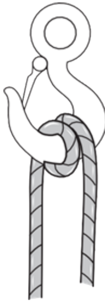
Figure 9 Never wrap a hook (BC Industry Training Authority, 2019). CC BY-NC-SA 4.0 ( https://creativecommons.org/licenses/by-nc-sa/4.0/ )
