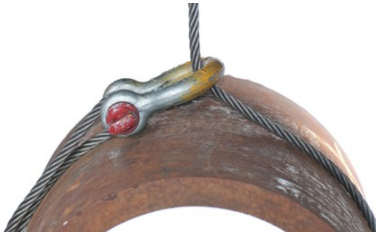
Figure 11 Using a shackle for a choker hitch (BC Industry Training Authority, 2019). CC BY-NC-SA 4.0 ( https://creativecommons.org/licenses/by-nc-sa/4.0/ )
