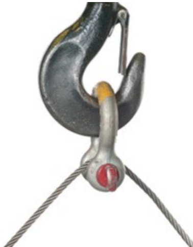
Figure 9 Incorrect shackle attachment (BC Industry Training Authority, 2019). CC BY-NC-SA 4.0 ( https://creativecommons.org/licenses/by-nc-sa/4.0/ )
