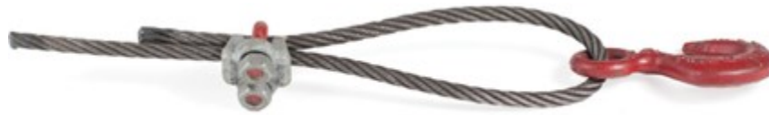
Figure 14 Installing first cable clip (BC Industry Training Authority, 2019). CC BY-NC-SA 4.0 ( https://creativecommons.org/licenses/by-nc-sa/4.0/ )
