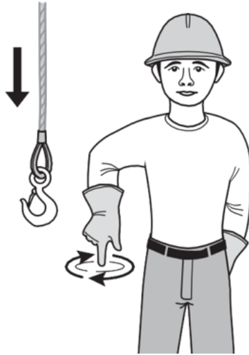
Figure 3 Lower the load (BC Industry Training Authority, 2019). CC BY-NC-SA 4.0 ( https://creativecommons.org/licenses/by-nc-sa/4.0/ )
