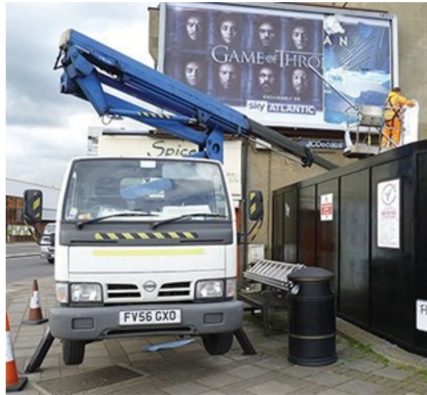
Figure 5 Boom truck with outriggers (PhilaFrenzy/Wikimedia Commons) CC BY-SA 4.0 ( https://creativecommons.org/licenses/by-sa/4.0/deed.en )
