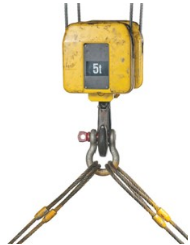
Figure 8 Wire ropes on shackle over hook (BC Industry Training Authority, 2019). CC BY-NC-SA 4.0 ( https://creativecommons.org/licenses/by-nc-sa/4.0/ )
