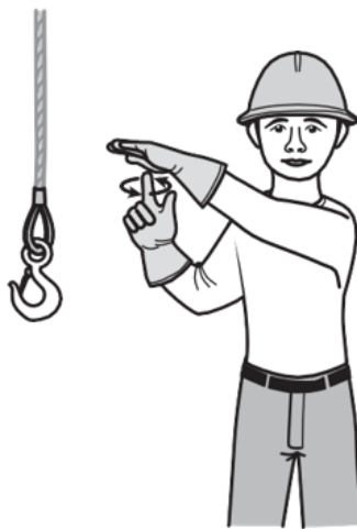
Figure 11 Raise the load-slowly (BC Industry Training Authority, 2019). CC BY-NC-SA 4.0 ( https://creativecommons.org/licenses/by-nc-sa/4.0/ )
