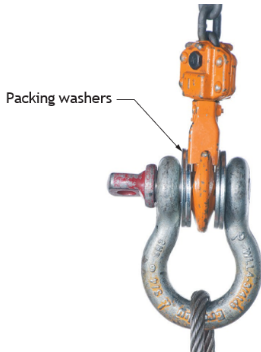
Figure 10 Apply load to pin (BC Industry Training Authority, 2019). CC BY-NC-SA 4.0 ( https://creativecommons.org/licenses/by-nc-sa/4.0/ )
