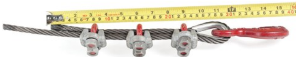
Figure 16 Installing centre cable clips (BC Industry Training Authority, 2019). CC BY-NC-SA 4.0 ( https://creativecommons.org/licenses/by-nc-sa/4.0/ )
