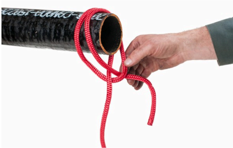
Figure 18 Clove hitch pre-tied to slip over end of pipe (Camosun College/BCcampus). CC BY-NC-SA 4.0 ( https://creativecommons.org/licenses/by-nc-sa/4.0/ )
