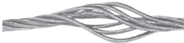
Figure 2 “Bird caging” (BC Industry Training Authority, 2019). CC BY-NC-SA 4.0 ( https://creativecommons.org/licenses/by-nc-sa/4.0/ )
