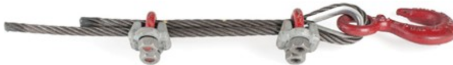
Figure 15 Installing second cable clip (BC Industry Training Authority, 2019). CC BY-NC-SA 4.0 ( https://creativecommons.org/licenses/by-nc-sa/4.0/ )
