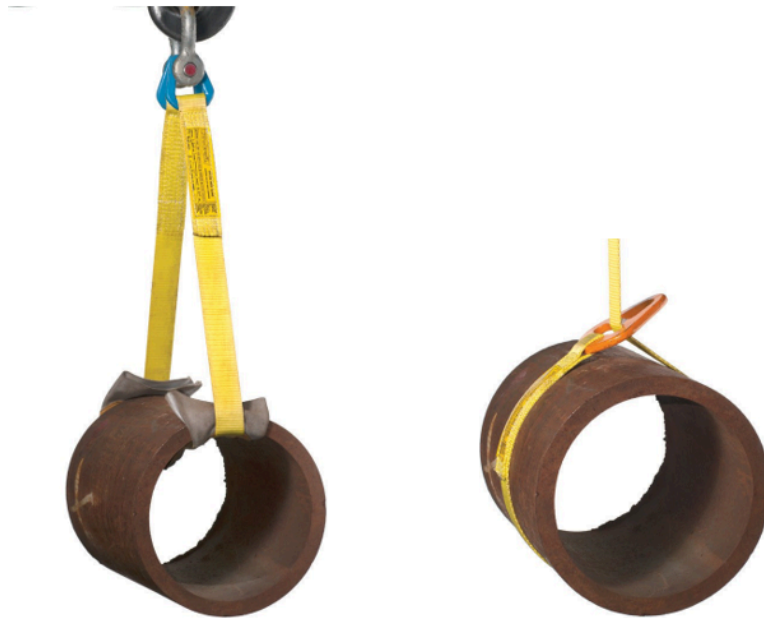
Figure 24 (left) Basket web sling (right) choker web sling (BC Industry Training Authority, 2019). CC BY-NC-SA 4.0 ( https://creativecommons.org/licenses/by-nc-sa/4.0/ )
