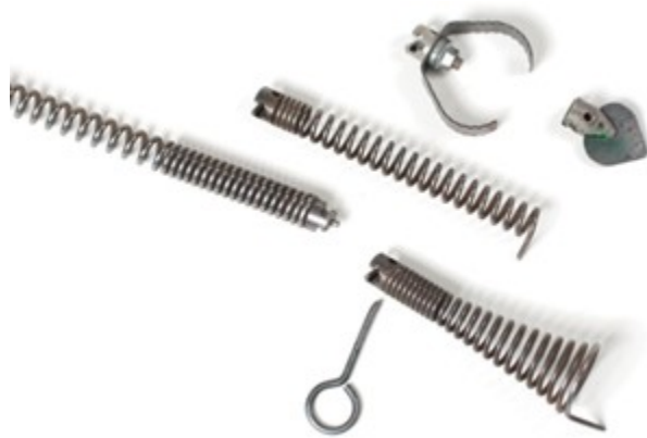
Figure 59 Sections of drain auger (snake) and common head attachments (BC Industry Training Authority, 2019). CC BY-NC-SA 4.0 ( https://creativecommons.org/licenses/by-nc-sa/4.0/ )
