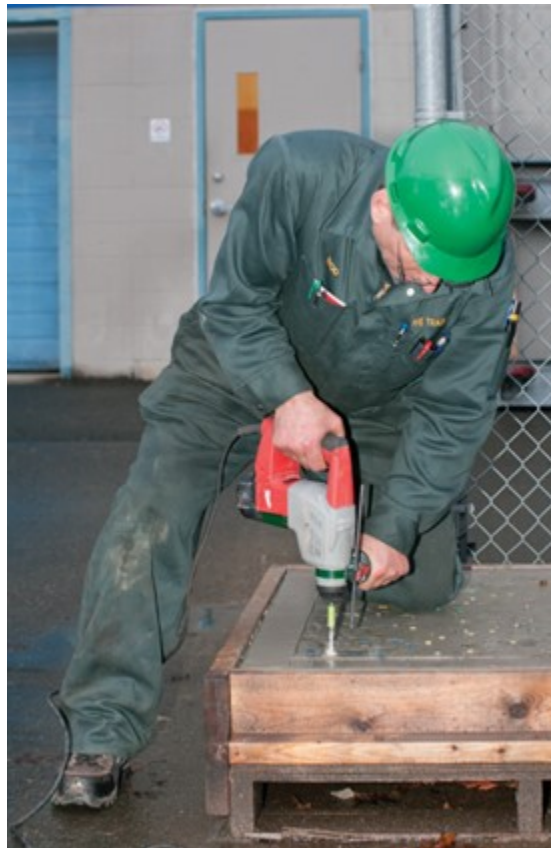
Figure 13 Using a hammer drill (BC Industry Training Authority, 2019). CC BY-NC-SA 4.0 ( https://creativecommons.org/licenses/by-nc-sa/4.0/ )
