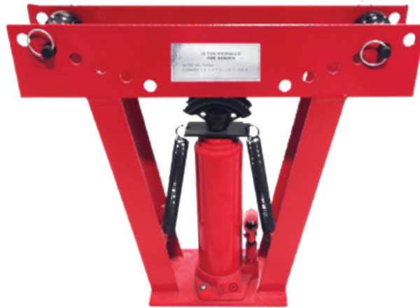
Figure 26 Portable Hydraulic Tube and Pipe Bender (BC Industry Training Authority, 2019). CC BY-NC-SA 4.0 ( https://creativecommons.org/licenses/by-nc-sa/4.0/ )
