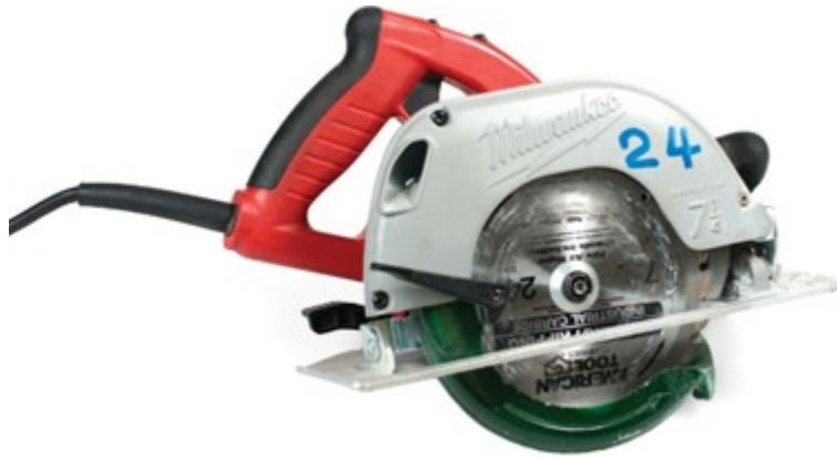
Figure 1 Electric portable circular saw (BC Industry Training Authority, 2019). CC BY-NC-SA 4.0 ( https://creativecommons.org/licenses/by-nc-sa/4.0/ )
