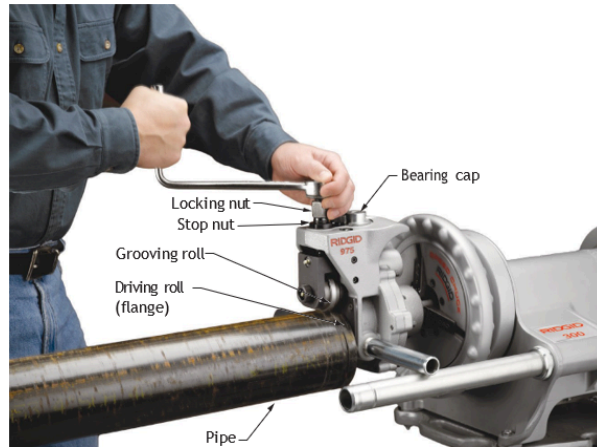
Figure 35 Feeding grooving roll into pipe with hand wheel (BC Industry Training Authority, 2019). CC BY-NC-SA 4.0 ( https://creativecommons.org/licenses/by-nc-sa/4.0/ )
