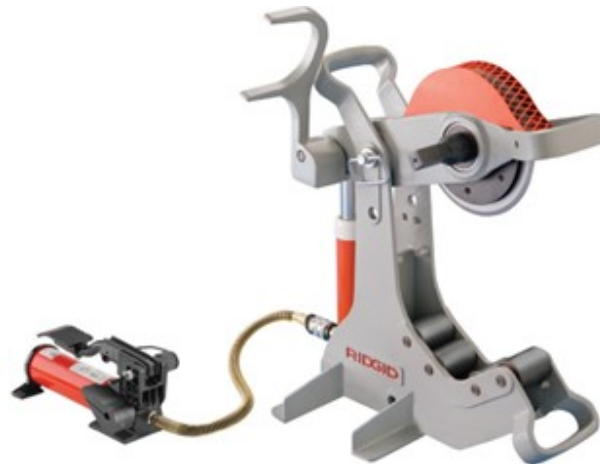
Figure 44 Power pipe cutter (RIDGID TOOLS/Emerson Professional Tools) Used with permission.
