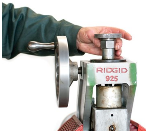
Figure 34 Adjusting the stop nut/feed screw on the Model 925 (BC Industry Training Authority, 2019). CC BY-NC-SA 4.0 ( https://creativecommons.org/licenses/by-nc-sa/4.0/ )
