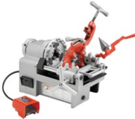
Figure 17 Ridgid Model 1210 Oil-Free Compact Threading Machine (RIDGID TOOLS/Emerson Professional Tools) Used with permission.
