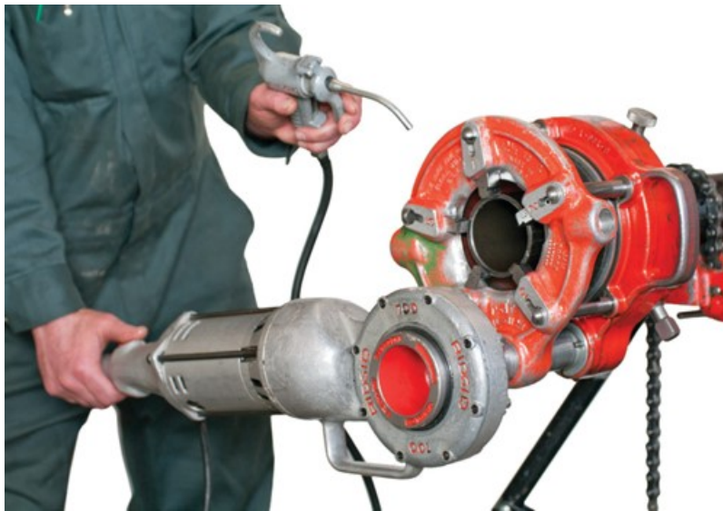
Figure 19 Using the portable power drive with the geared threader (BC Industry Training Authority, 2019). CC BY-NC-SA 4.0 ( https://creativecommons.org/licenses/by-nc-sa/4.0/ )
