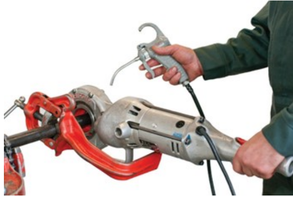
Figure 43 Threading with a portable power drive using a support arm (BC Industry Training Authority, 2019). CC BY-NC-SA 4.0 ( https://creativecommons.org/licenses/by-nc-sa/4.0/ )
