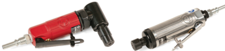
Figure 67 Typical heavy duty air-operated grinders (BC Industry Training Authority, 2019). CC BY-NC-SA 4.0 ( https://creativecommons.org/licenses/by-nc-sa/4.0/ )
