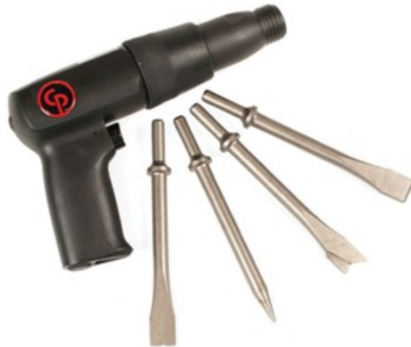
Figure 69 Air-operated hammer/chisel (BC Industry Training Authority, 2019). CC BY-NC-SA 4.0 ( https://creativecommons.org/licenses/by-nc-sa/4.0/ )
