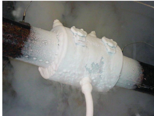
Figure 63 Electric pipe freeze kit and a frozen pipe (RIDGID TOOLS/Emerson Professional Tools) Used with permission.
