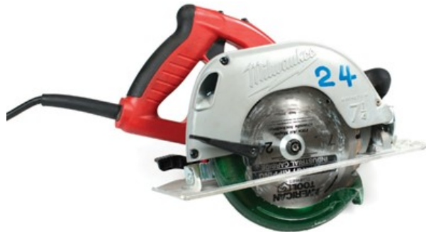
Figure 2 Portable electric circular saw (BC Industry Training Authority, 2019). CC BY-NC-SA 4.0 ( https://creativecommons.org/licenses/by-nc-sa/4.0/ )
