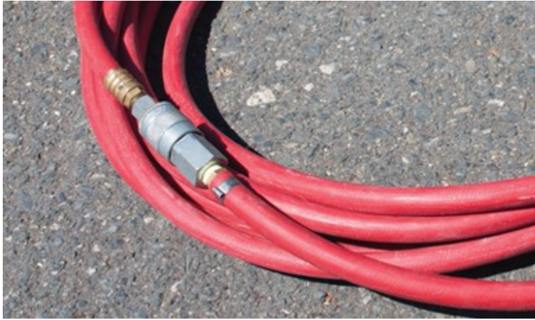
Figure 20 Store hose with ends connected (BC Industry Training Authority, 2019). CC BY-NC-SA 4.0 ( https://creativecommons.org/licenses/by-nc-sa/4.0/ )
