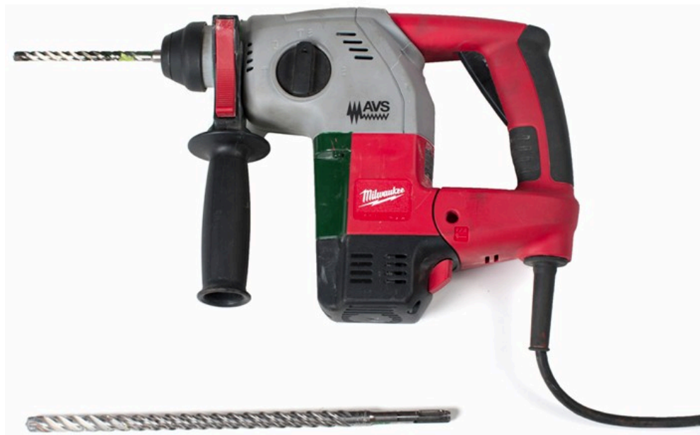
Figure 31 Hammer drill (roto-hammer) and masonry bits (BC Industry Training Authority, 2019). CC BY-NC-SA 4.0 ( https://creativecommons.org/licenses/by-nc-sa/4.0/ )
