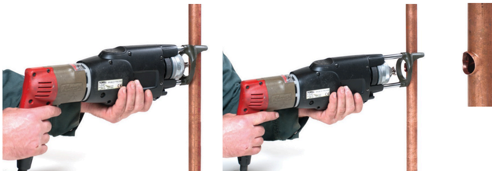
Figure 36 Extracted-tee drill motor and branch outlets (BC Industry Training Authority, 2019). CC BY-NC-SA 4.0 ( https://creativecommons.org/licenses/by-nc-sa/4.0/ )
