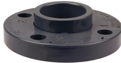
Socket flange S, PVC Schedule 80, two-piece van stone (Courtesy of NIBCO INC)
