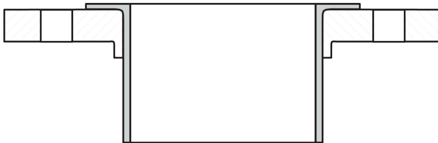
Figure 62 300 psi lap joint flange (BC Industry Training Authority, 2019). CC BY-NC-SA 4.0 ( https://creativecommons.org/licenses/by-nc-sa/4.0/ )
