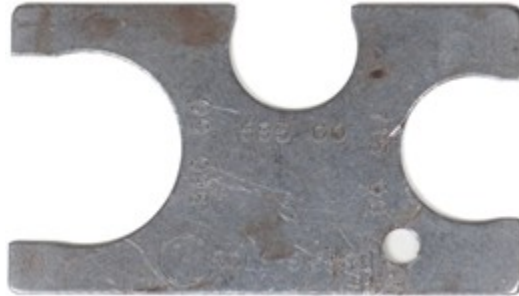
Figure 99 Go/no-go gauge (BC Industry Training Authority, 2019). CC BY-NC-SA 4.0 ( https://creativecommons.org/licenses/by-nc-sa/4.0/ )
