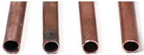
Figure 43 Examine pipe ends for damage (BC Industry Training Authority, 2019). CC BY-NC-SA 4.0 ( https://creativecommons.org/licenses/by-nc-sa/4.0/ )
