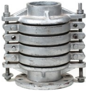
Figure 18 Bellows-type expansion joint with shipping bars. (Do not remove bars until after installation.) (BC Industry Training Authority, 2019). CC BY-NC-SA 4.0 ( https://creativecommons.org/licenses/by-nc-sa/4.0/ )
