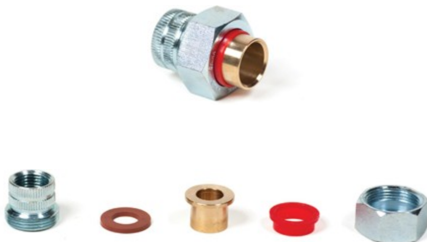
Figure 46 Dielectric union (BC Industry Training Authority, 2019). CC BY-NC-SA 4.0 ( https://creativecommons.org/licenses/by-nc-sa/4.0/ )
