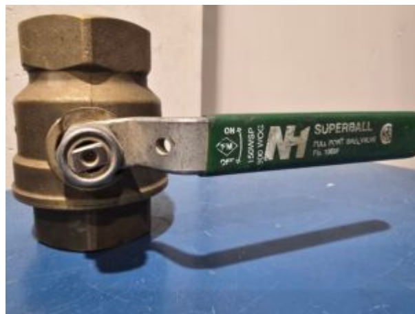
Figure 7b Example letter code on a crane valve (Audrey Curran/TRU Open Press) CC BY-NC-SA ( https://creativecommons.org/licenses/by-nc-sa/4.0/deed.en )
