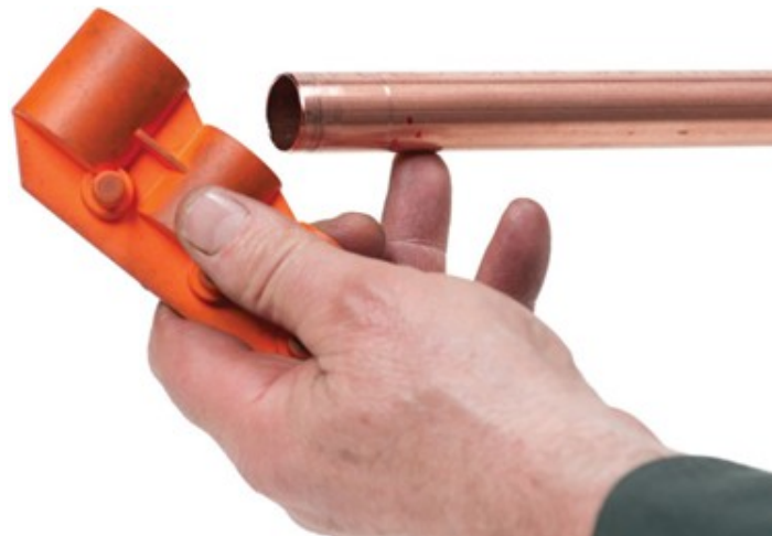
Figure 45 Chamfered OD of tube (BC Industry Training Authority, 2019). CC BY-NC-SA 4.0 ( https://creativecommons.org/licenses/by-nc-sa/4.0/ )
