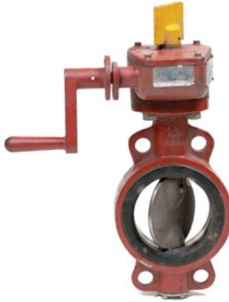
Figure 38 Wafer lug type butterfly valve. No gaskets required; manual gear operated; indicator for fire service (BC Industry Training Authority, 2019). CC BY-NC-SA 4.0 ( https://creativecommons.org/licenses/by-nc-sa/4.0/ )
