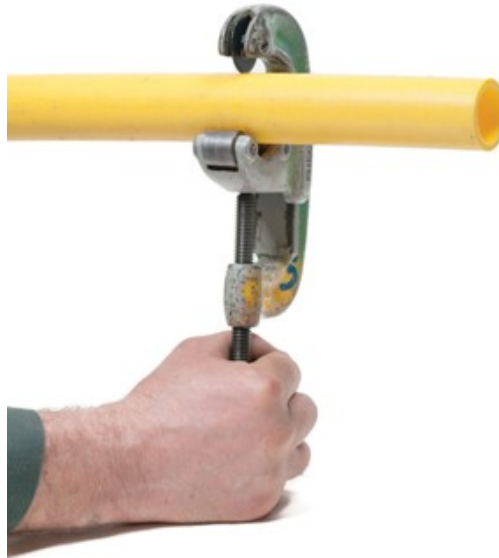
Figure 64 A regular plastic pipe cutter with a plastic cutter wheel can be used to cut the pipe (BC Industry Training Authority, 2019). CC BY-NC-SA 4.0 ( https://creativecommons.org/licenses/by-nc-sa/4.0/ )
