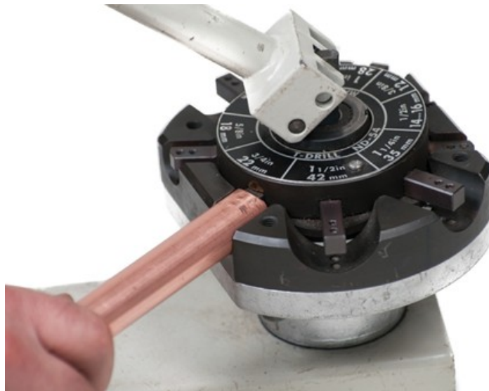
Figure 36 Using the notching and dimpling tool (BC Industry Training Authority, 2019). CC BY-NC-SA 4.0 ( https://creativecommons.org/licenses/by-nc-sa/4.0/ )
