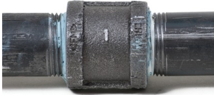
Figure 90 Correctly threaded joint (BC Industry Training Authority, 2019). CC BY-NC-SA 4.0 ( https://creativecommons.org/licenses/by-nc-sa/4.0/ )
