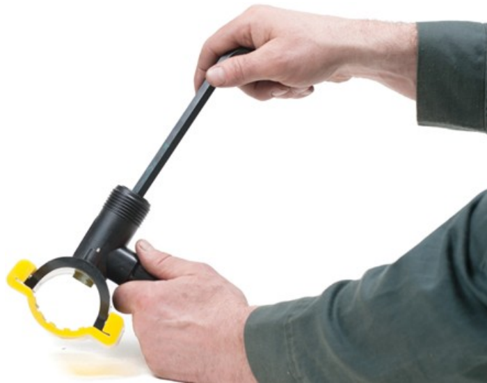
Figure 80 Cap removed to show cutter head (BC Industry Training Authority, 2019). CC BY-NC-SA 4.0 ( https://creativecommons.org/licenses/by-nc-sa/4.0/ )
