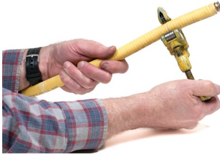
Figure 108 Cut the pipe (BC Industry Training Authority, 2019). CC BY-NC-SA 4.0 ( https://creativecommons.org/licenses/by-nc-sa/4.0/ )
