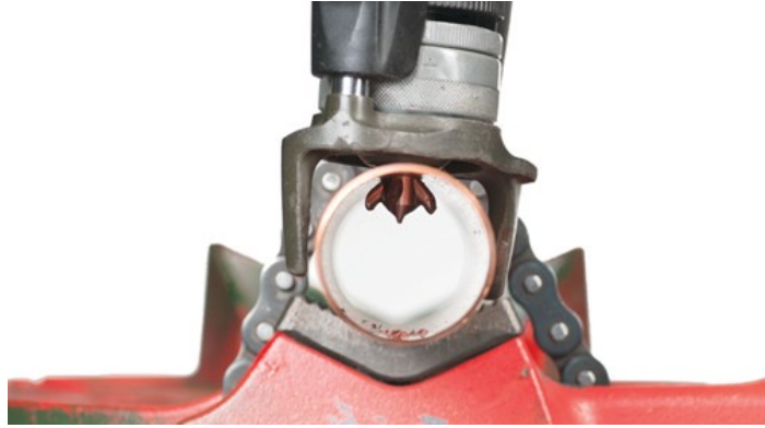
Figure 33 Stop drill and extend the forming pins (BC Industry Training Authority, 2019). CC BY-NC-SA 4.0 ( https://creativecommons.org/licenses/by-nc-sa/4.0/ )
