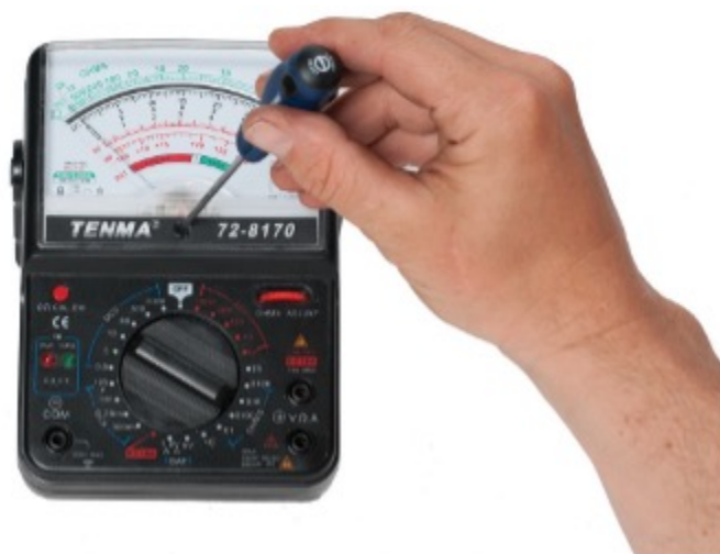
Figure 3 Mechanical adjustment of the zero reading (BC Industry Training Authority, 2019). CC BY-NC-SA 4.0
