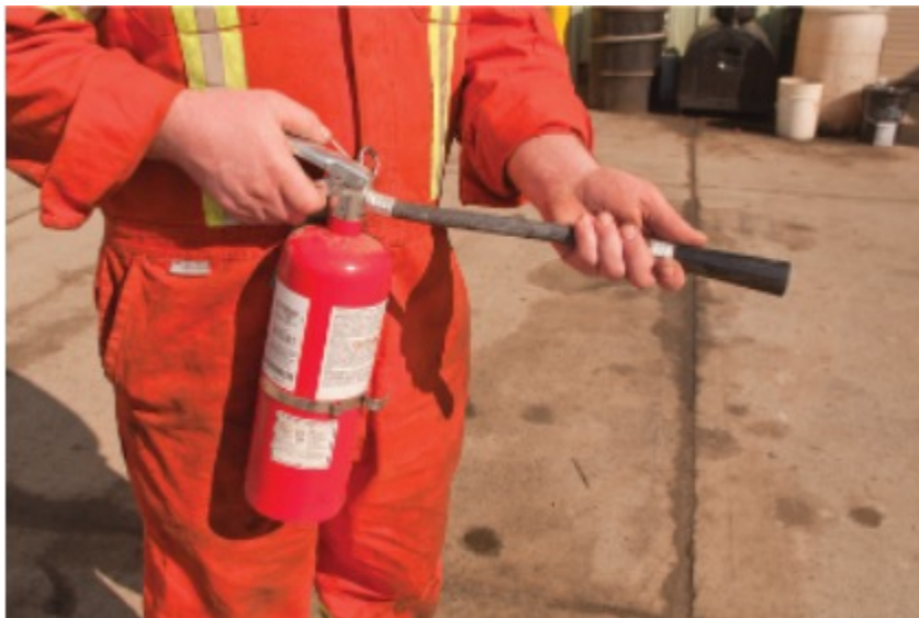
Figure 2 Aim the nozzle (BC Industry Training Authority, 2019). CC BY-NC-SA 4.0 ( https://creativecommons.org/licenses/by-nc-sa/4.0/ )
