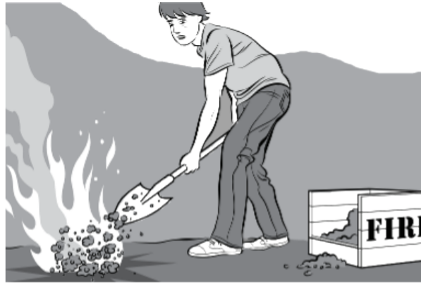
Figure 2 Extinguishing powder applied by shovel or scoop (BC Industry Training Authority, 2019). CC BY-NC-SA 4.0 ( https://creativecommons.org/licenses/by-nc-sa/4.0/ )
