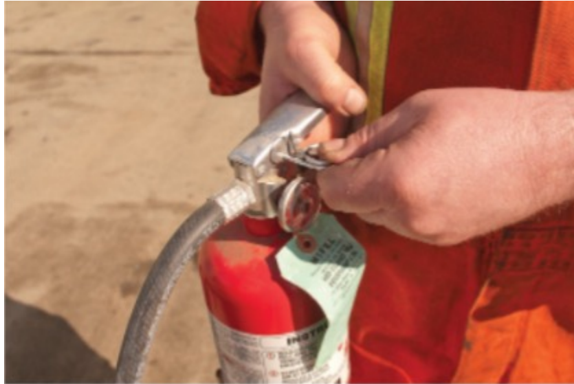
Figure 1 Pull the pin (BC Industry Training Authority, 2019). CC BY-NC-SA 4.0 ( https://creativecommons.org/licenses/by-nc-sa/4.0/ )
