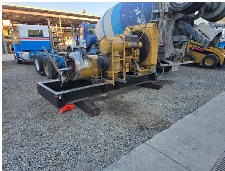
Figure 4a. Heavy equipment stabilized using timber support blocks placed beneath the frame on level gravel to prevent downward movement. (Audrey Curran/TRU Open Press) CC BY-NC-SA 4.0 ( https://creativecommons.org/licenses/by-nc-sa/4.0/ )
