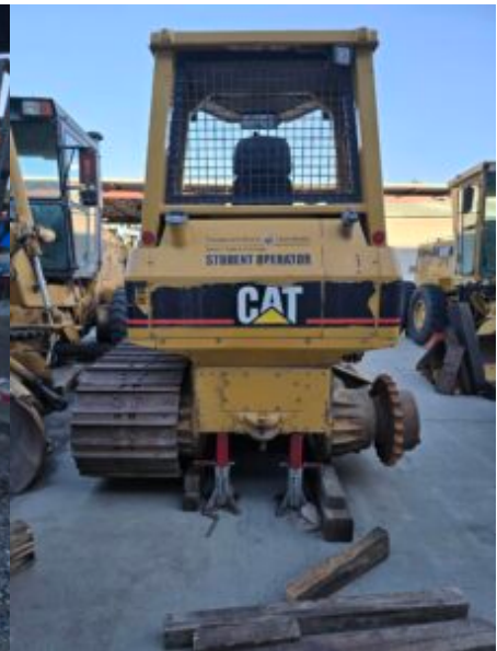
Figure 4c. Tracked equipment supported with blocking beneath the chassis to prevent movement while components are removed. (Audrey Curran/TRU Open Press) CC BY-NC-SA 4.0 ( https://creativecommons.org/licenses/by-nc-sa/4.0/ )
