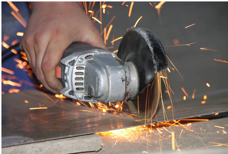
Figure 3 Cutting iron with a metal cutting machine (byrev/rawpixel) CC0 license ( https://creativecommons.org/publicdomain/zero/1.0/ ).
